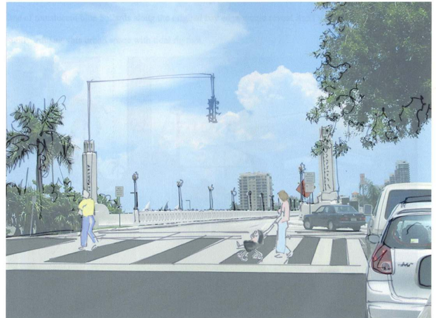
Figure 27. Sketch of proposed traffic light and pedestrian grade crosswalk at Venetian Causeway.
