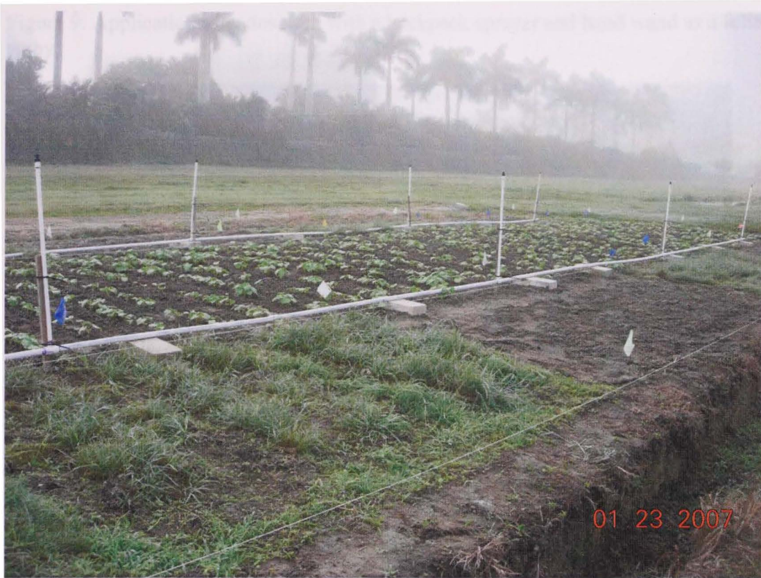
Figure 7: Test plot with the switchgrass buffer strip (left) and strip of bare soil (right).
