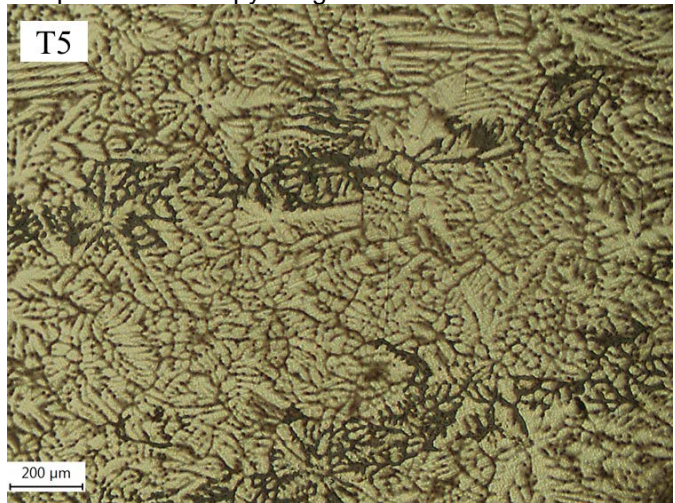
Figure 4.7. Optical microscopy images of T5 and Ti modified as cast alloys
