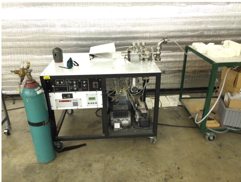
Figure 3.2. Custom-made vacuum set-up for encapsulation
