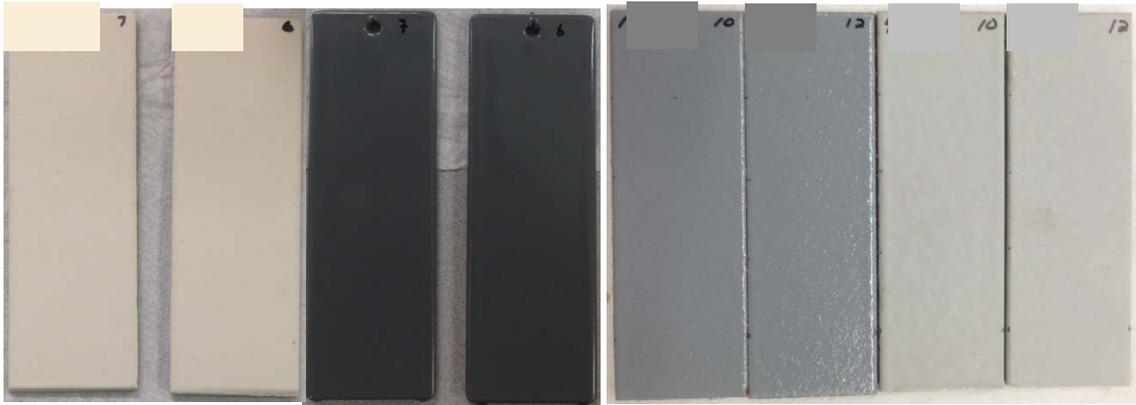
Figure 31: Phenolic Epoxy & FBE as received.
