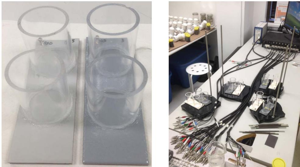
Figure 25: Acrylic tubes glued on coated panels
