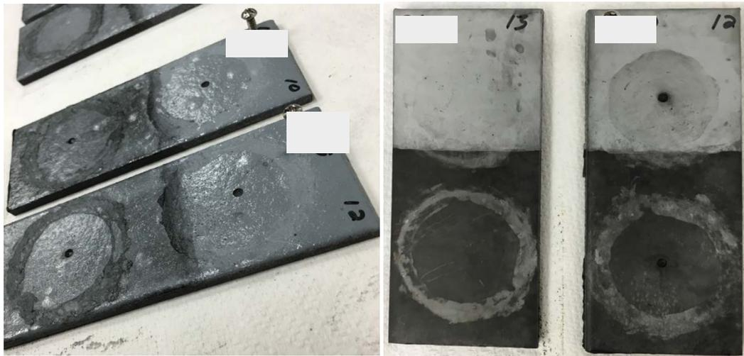
Figure 46: Amine Novolac and Novolac Epoxy coated panels after the autoclave test.
