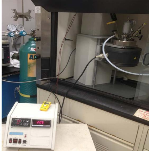
Figure 29: Parr Bench Top Reactor and Temperature Controller.
