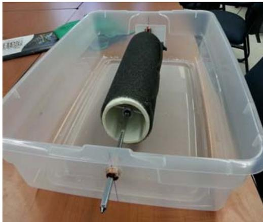
Figure 8. Semi-Submerged, Rotary System
