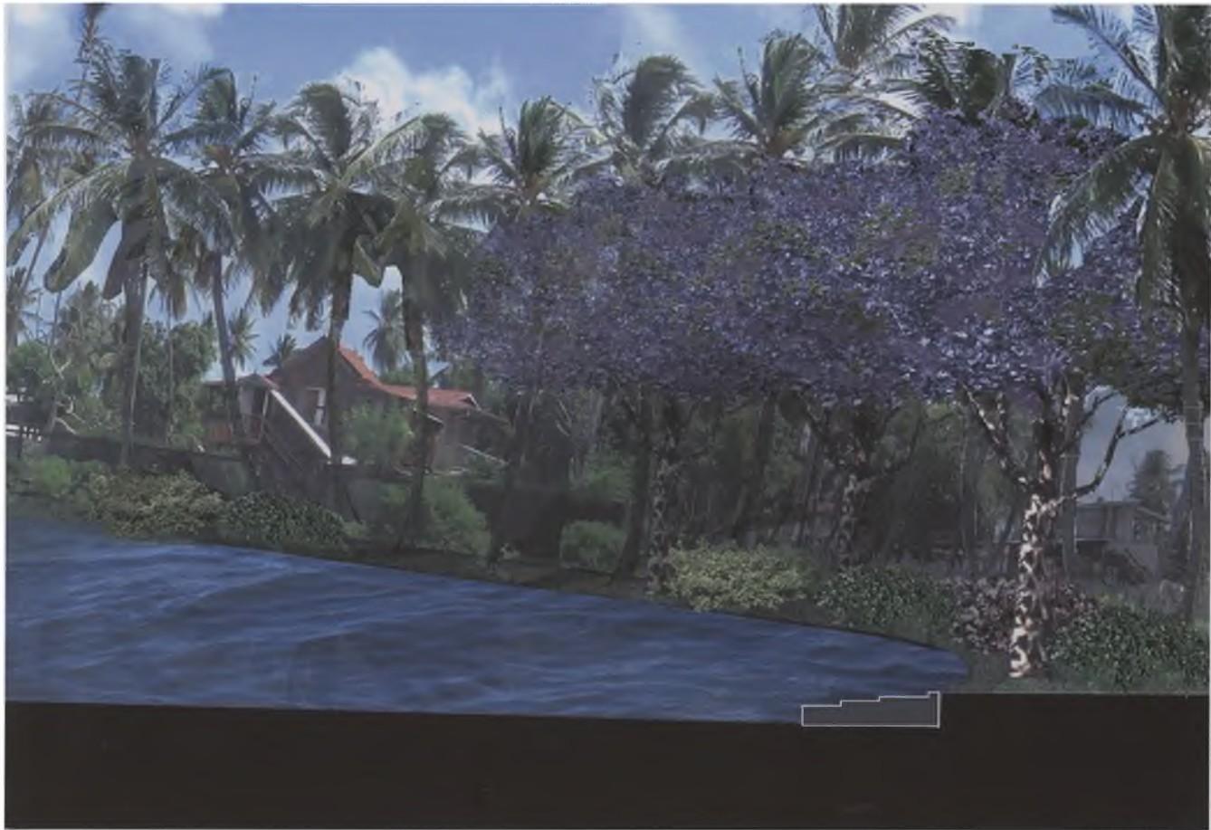
Figure 43: Sectional Study AA of Flood Plain—Rainy Season. The slope in the field will allow water to accumulate and slowly drain into the existing Village irrigation system. This reduces the possibility of flooding.
