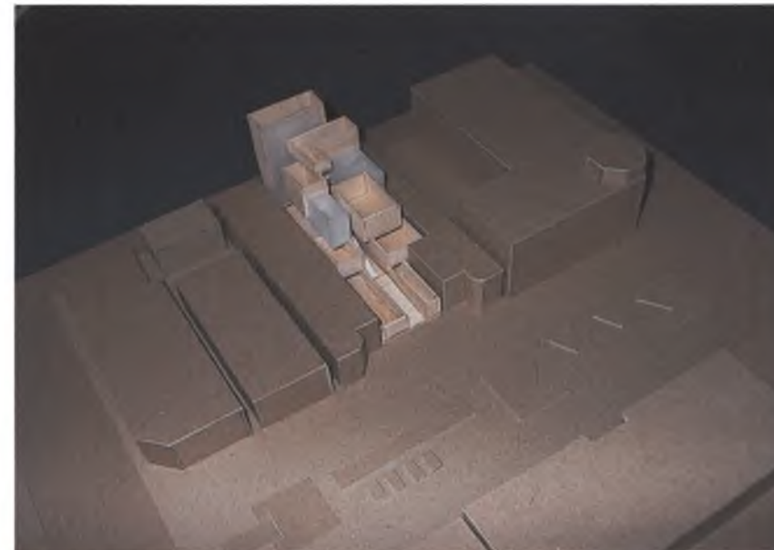
Figure 37 - Model for Terrace Design Concept. The model study shows how terracing provides greater privacy and power of observation to spaces at higher elevations. Narrowing of central connecting corridors and penetration of light further regulate the permeability of space.
