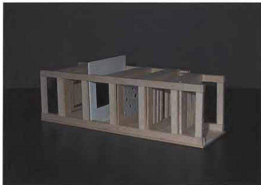
Figure 39 - Model for Curtain Design Concept. Model demonstrates how horizontal curtains visually define individual spaces within the gallery and their perception from the outside. The first curtains are more permeable to attract visitors to the gallery but become more restrictive in order to ensure privacy towards the rear of the structure.
