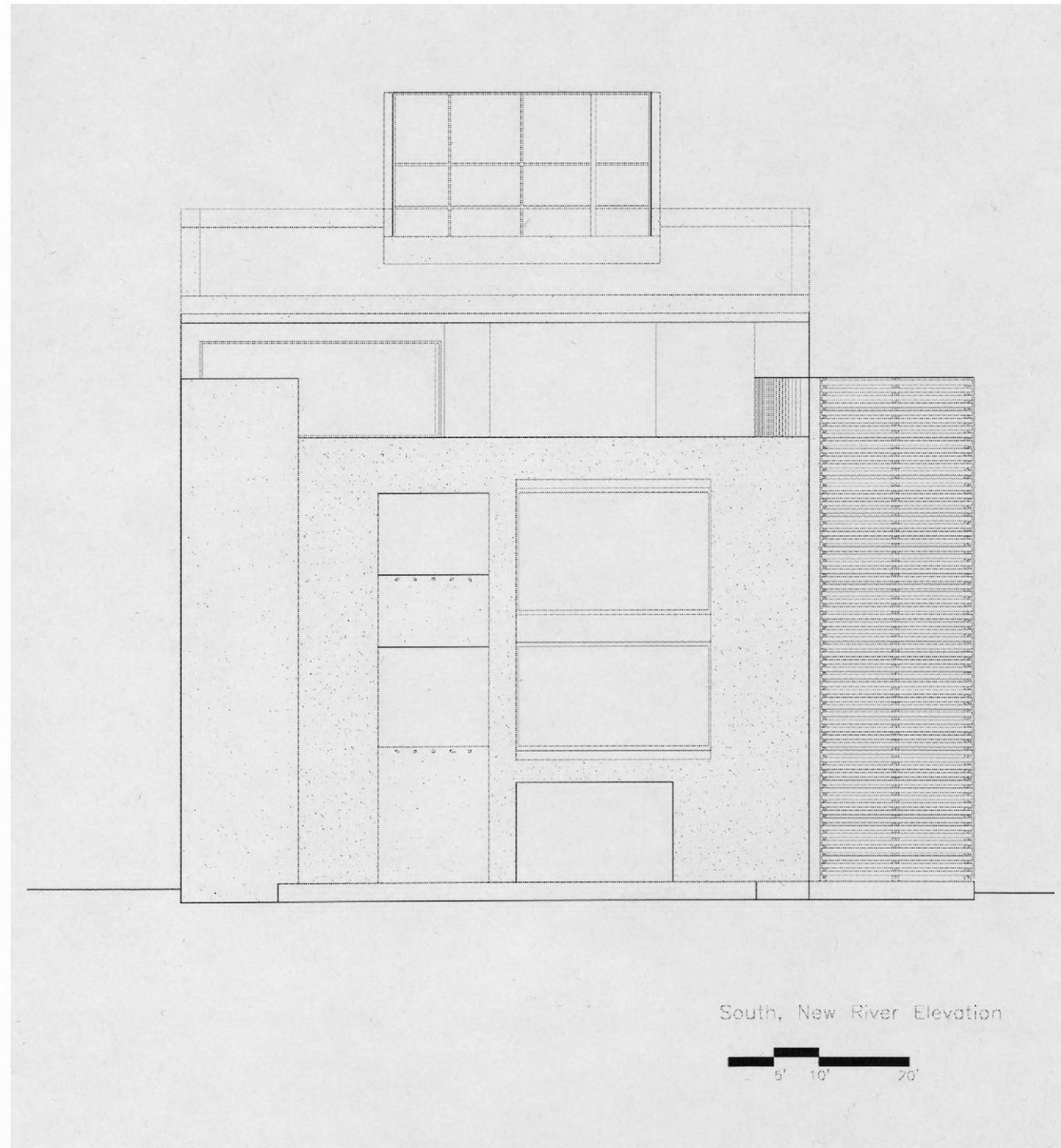
Figure 52 The south elevation faces the New River. A wall of water flows from the upper levels of the spa into the exercise pool.
