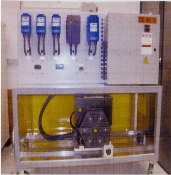
Figure 3.1-1 Generating station front panel
