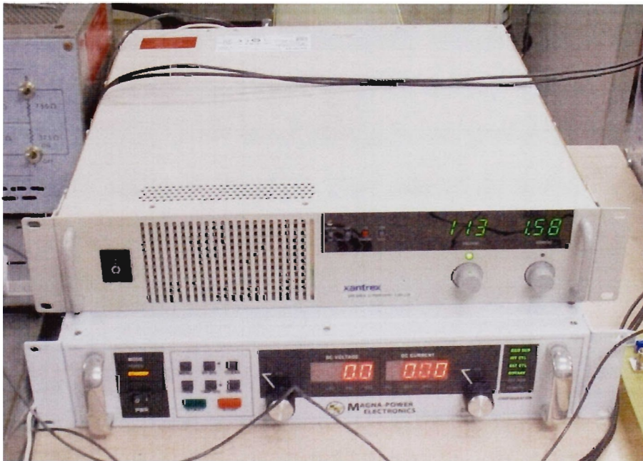
Figure 2.3-2 Fuel Cell Emulator from DC Power Supply
