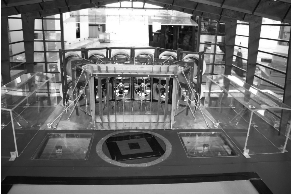
Figure 1. Small-Scale 12-Fan Wall-of-Wind (WoW)
