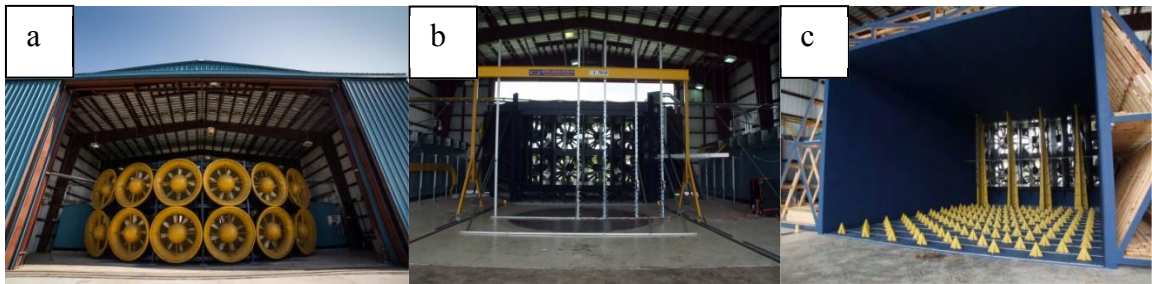
Figure 1. a. 12-Fan WOW Intake Side, b. WOW Exit Side Without Flow Management Devices, c. WOW Exit Side With Flow Management Devices
