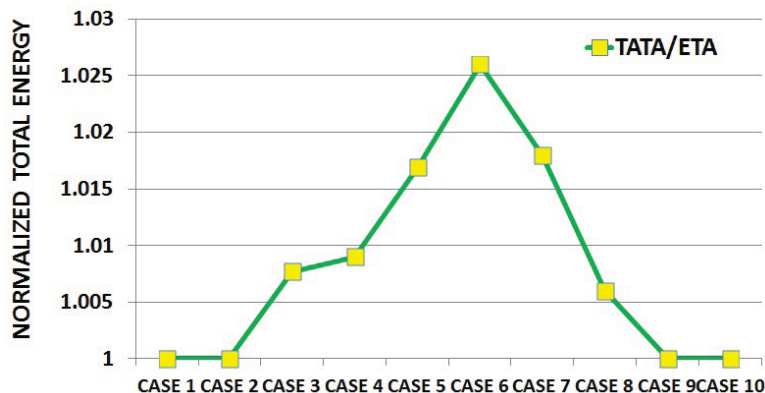
Figure 6.8: ETA-EM vs TATA-EM on 3x3 Multi-Core Platform
