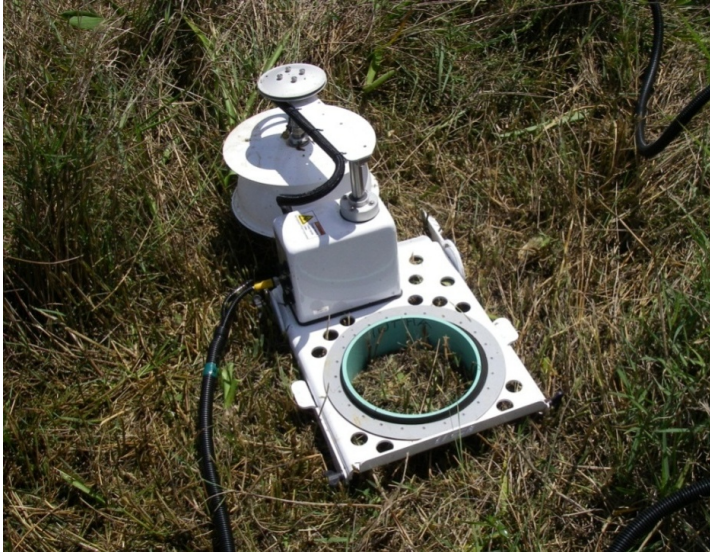
Figure 4. LICOR 20 cm PVC collar inserted into ground with a 104 long term chamber in open position.
