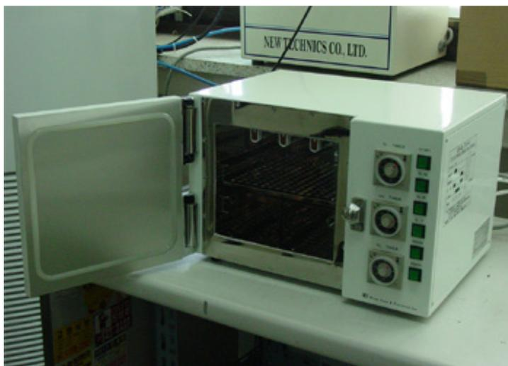
Figure 6.3. The actual UVy253 UV/O<sub>3</sub> surface pretreatment system
