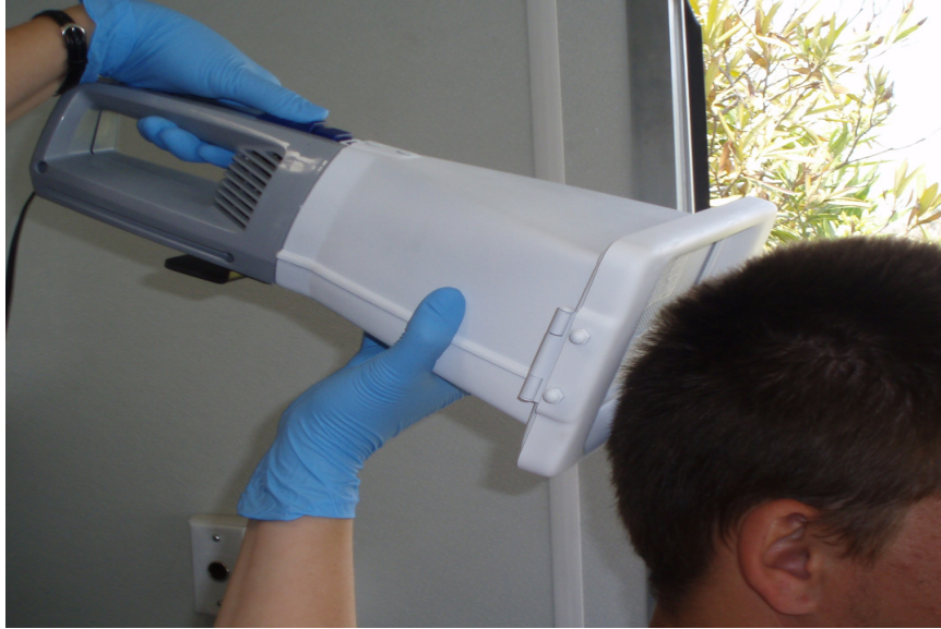
Figure 7-Scent Transfer Unit 100 (STU-100) collecting scent from head hair
