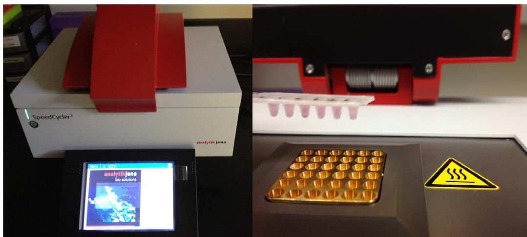
**Figure 59: The SpeedCycler<sup>2</sup><sup>®</sup> thermal cycler instrument shown on the left. The gold plated heated block and sample tubes shown on the right.**
