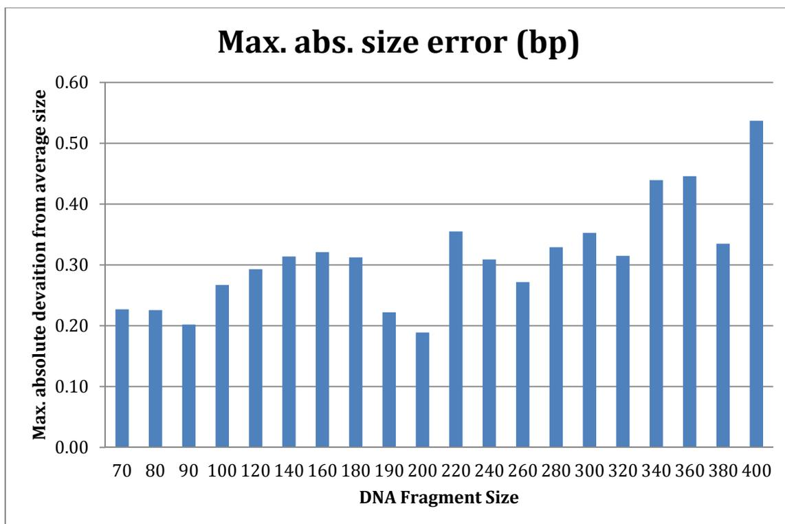
**Figure 50:** The maximum deviation from the calculated size to the actual size observed during the separation of a 400bp MapMarker<sup>®</sup> ladder on a 1.5cm separation channel microfluidic system. The average deviation is less than 0.3bp. The runs were performed with a separation voltage of 350V/cm with total run time of under 2minutes.
