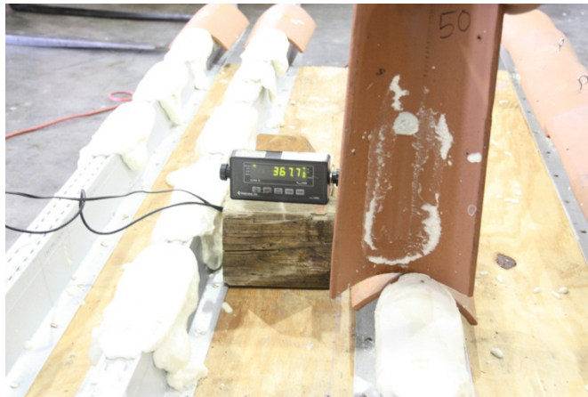
Figure 7.16: Bonding Failure at the Interface between Tile and Foam (Barrel tile)
