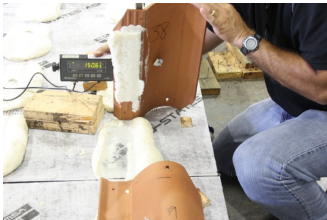
Figure 7.14: Failure within the Foam Paddy (Spanish 'S' tile)
