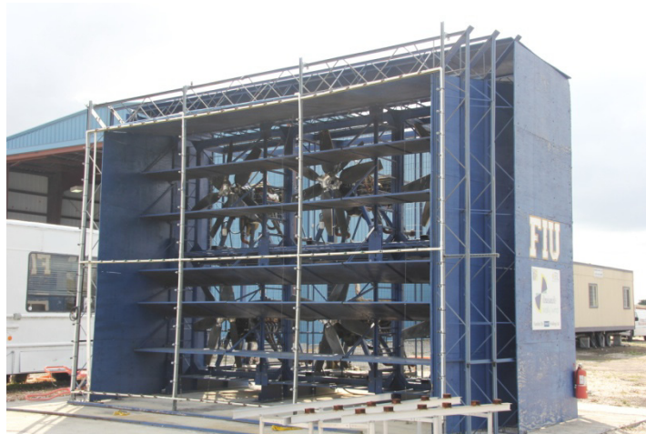
Figure 1.6: 6-fan Wall of Wind Testing Facility
