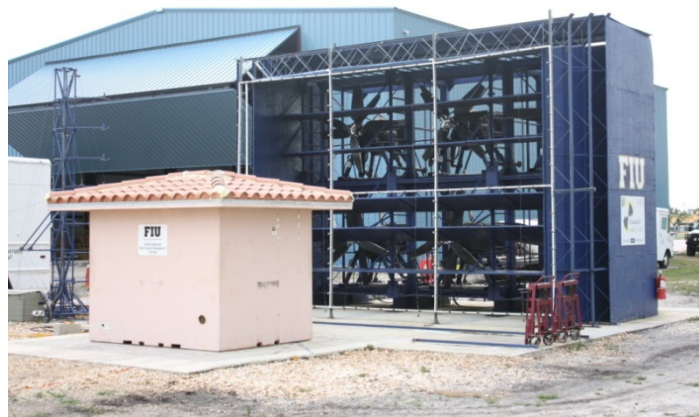
Figure 2.8: 6-fan Wall of Wind with a Testing Specimen
