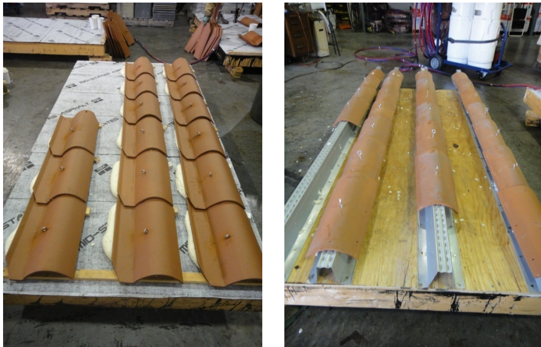
Figure 7.11: Tile Uplift Testing Specimens
