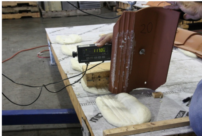
Figure 7.13: Bonding Failure at the Interface between Tile and Foam (Spanish 'S' tile)
