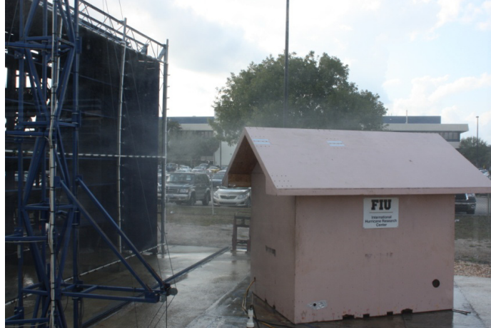
Figure 3.4: Wind-Driven Rain Simulation at 6-Fan Wow
