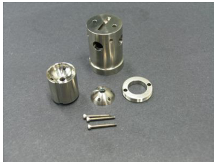
Figure 6-9 Diamod anvil cell made in CeSMEC machine shop
