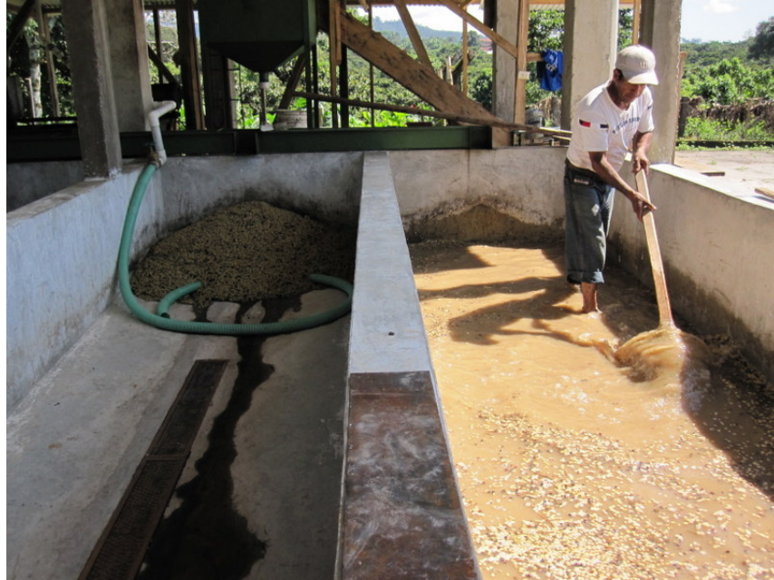
Figure 4.6 Beneficio work: pushing the depulped, fermented, and rinsed coffee beans into a flotation channel
