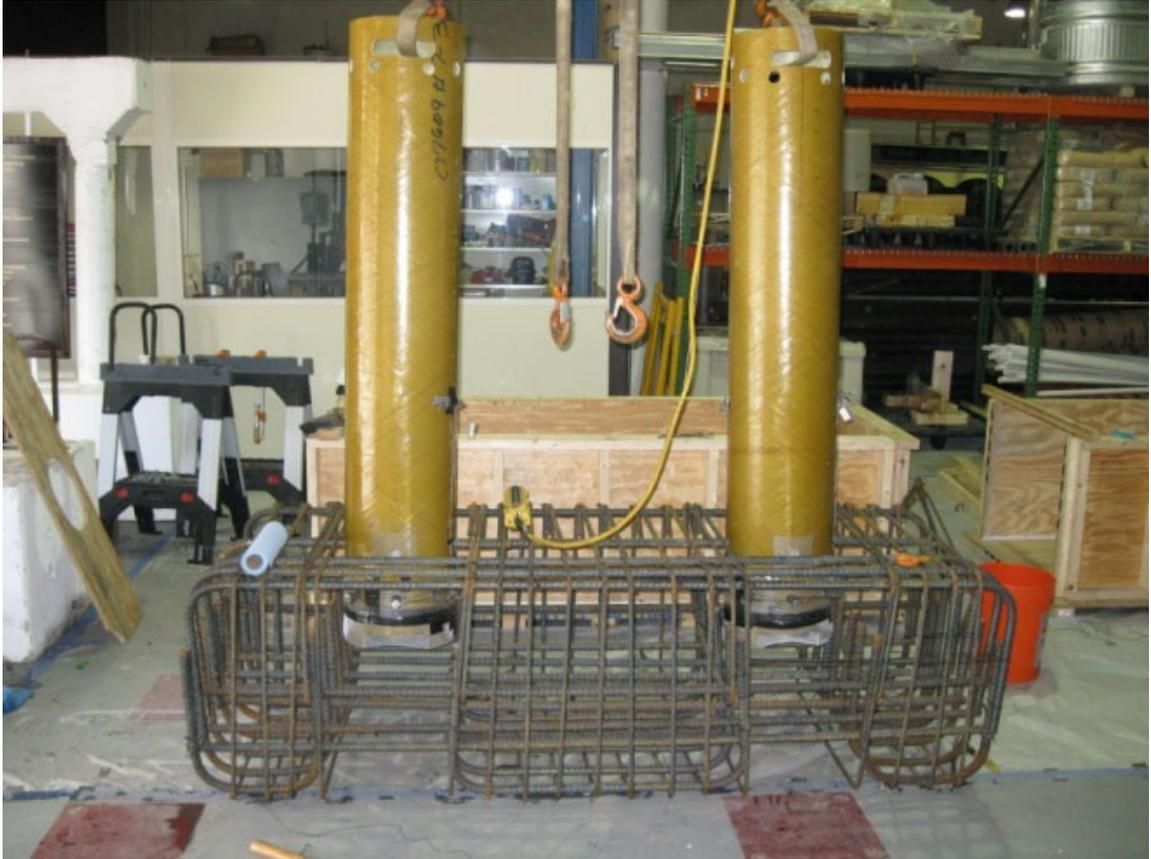
Figure 4.2 Embedded FRP Tubes for Specimens CFFT and UHPCFFT
