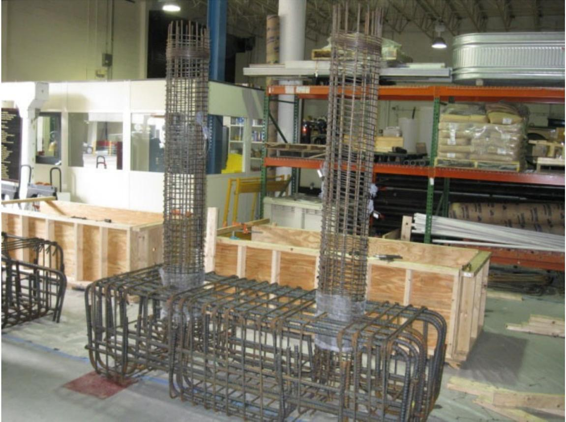
Figure 4.1 Reinforcement Cages for Specimens RC and RUHPC
