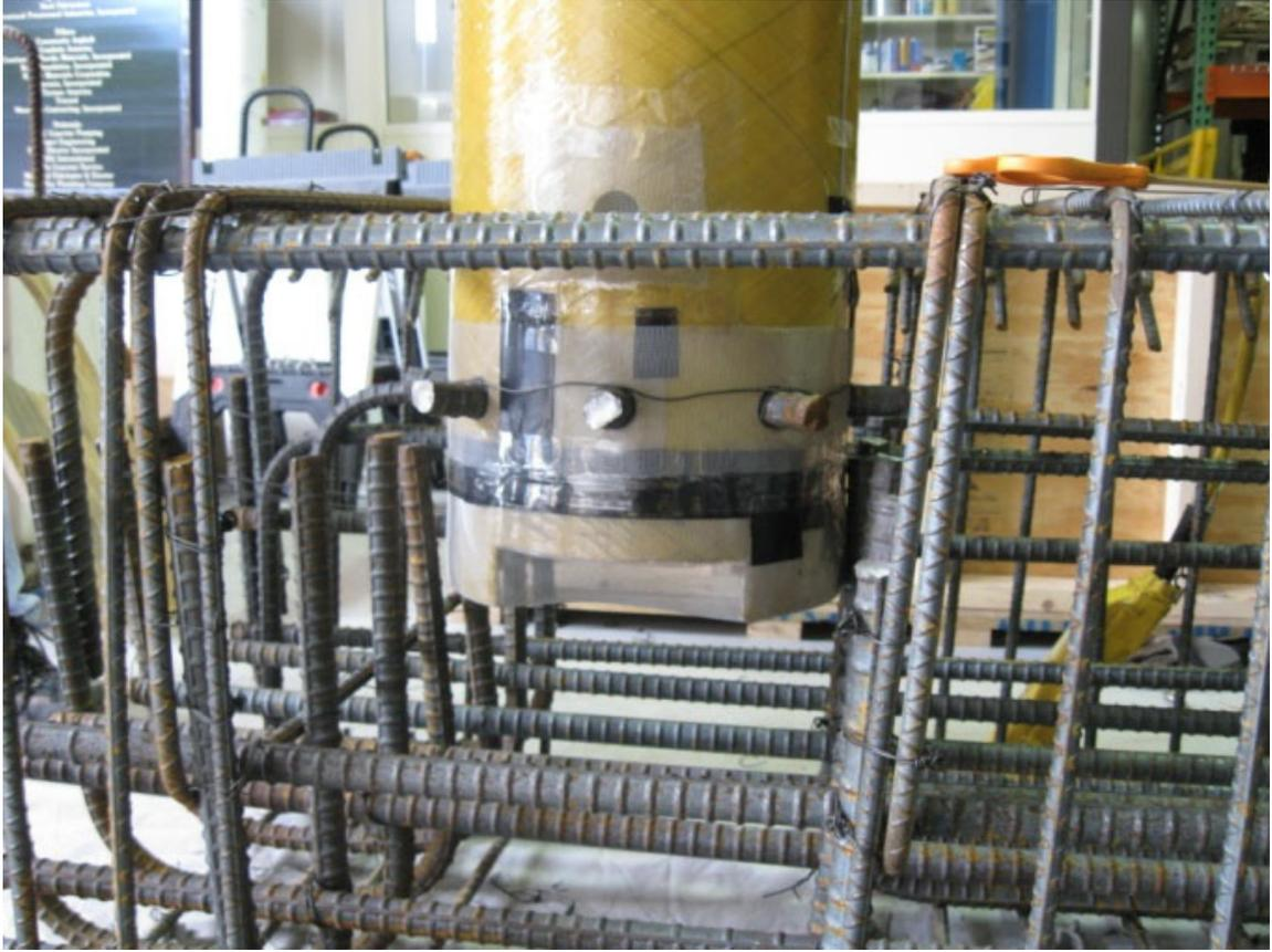
Figure 4.3 Shear Connectors and Screen at the Bottom of FRP Tube
