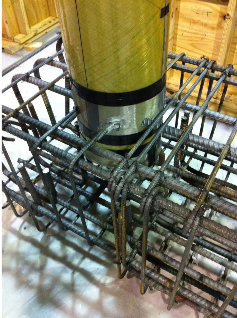
Figure 5.2 Embedment of FRP Tubes into the Footing
