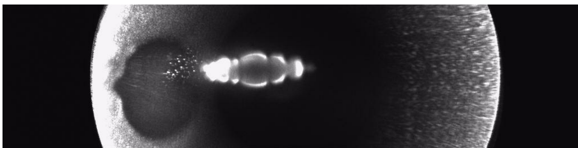
Figure 37. Aerosol LIBS effluent exiting the orifice into LIBS plasma
