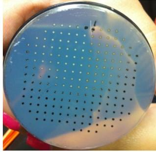
Figure 19: Optical detection fiber bundle of the Gen-2 imaging probe.
