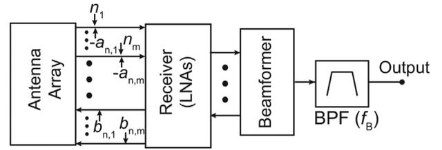
Fig. 1 Block diagram of the network
