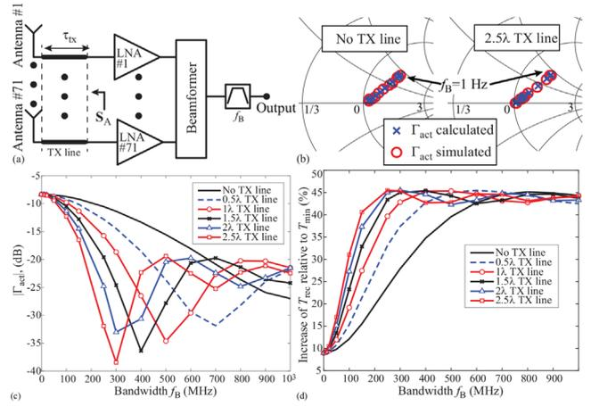
**Fig. 2** Simulated  $\Gamma_{\text{act}}$  and  $T_{\text{rec}}$  as a function of  $f_B$  of a 71-element Vivaldi antenna array operating at 1.4 GHz: (a) Block diagram with TX lines; (b)  $\Gamma_{\text{act}}$  as function of  $f_B$ ; (c)  $\Gamma_{\text{act}}$  [dB] as function of  $f_B$ ; and (d)  $T_{\text{rec}}$  as function of  $f_B$
