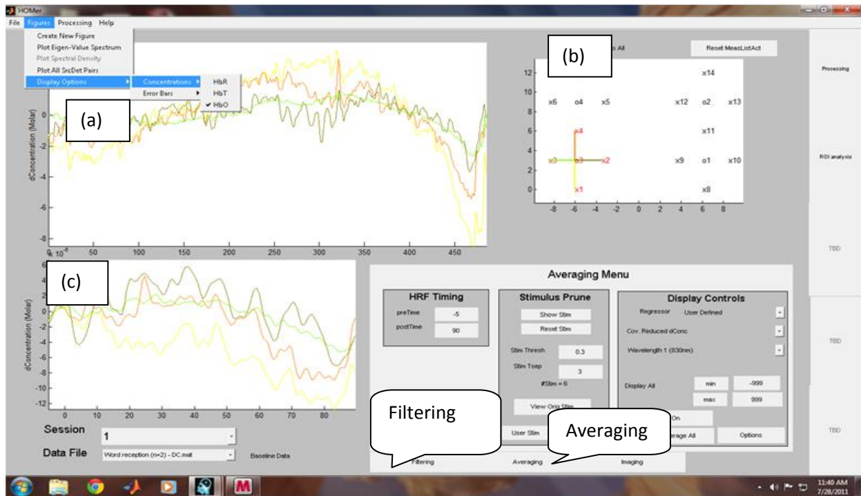
Figure 6. Screen shot of the HomER program. The layout of the HomER program is based around an interactive graphical display of the NIRS probe, shown in the upper right (b). The user specifies this probe geometry within the data file imported into HomER as described in the text. By selecting source (displayed as “x”) or detector (“o”) positions on this probe layout, the user navigates through the display of their data. The original data are shown in (a) and the average evoked response is shown in (c).
