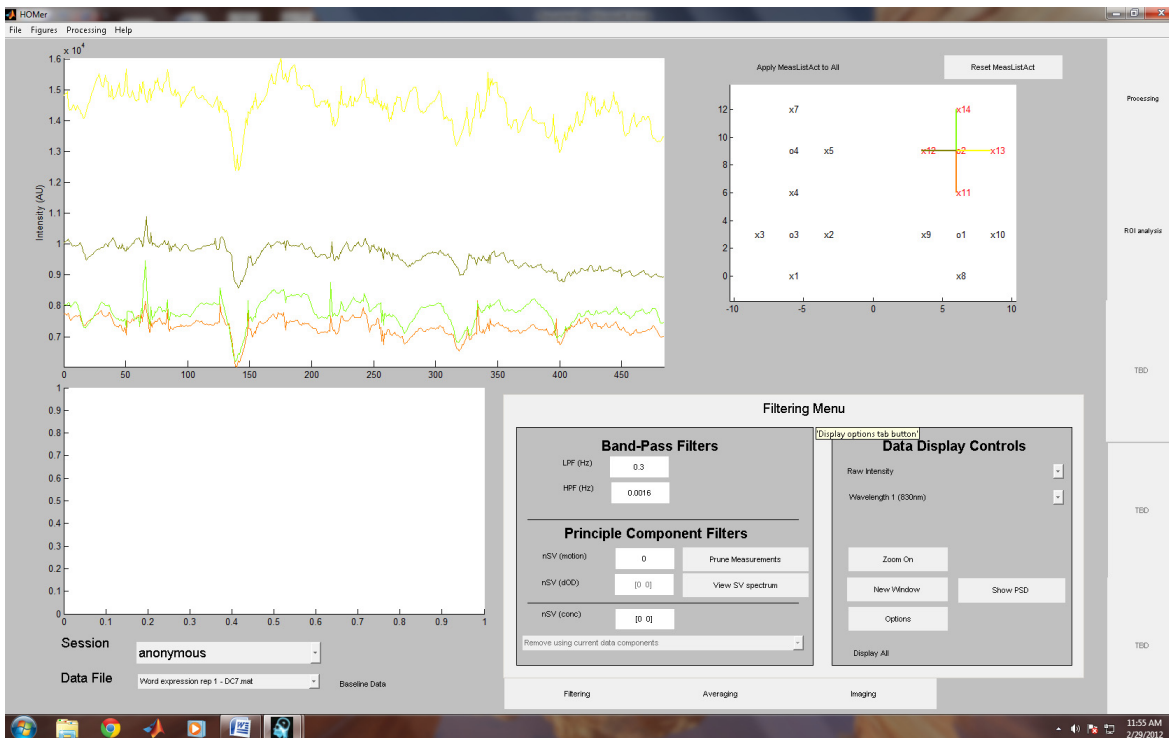
Figure B5. Figure showing HomER GUI interface with raw intensity signal after 3 rd order bandpass filtration for right anterior temporal region.
