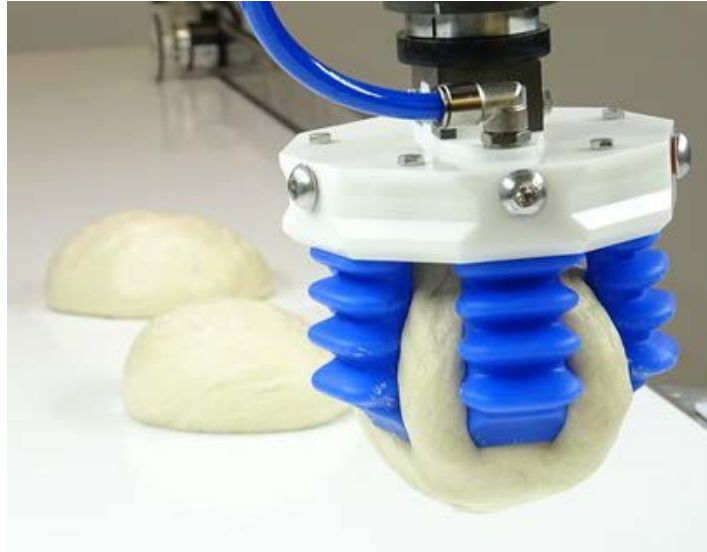
Figure 1: Industrial Robotic Gripper Picking Up Dough
