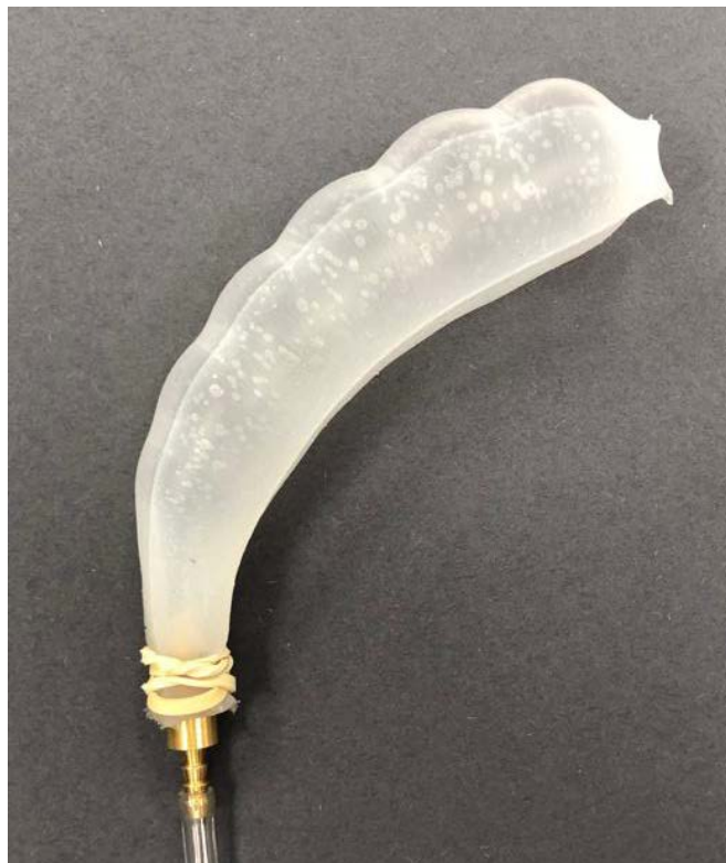
Figure 6: Casted Actuator Inflated
