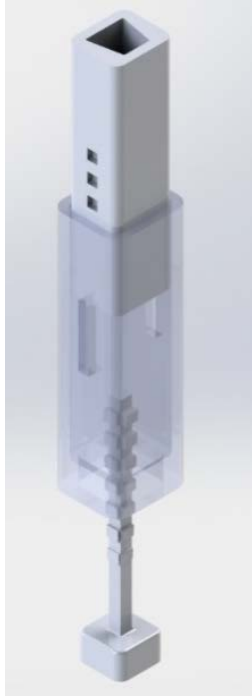
Figure 5: 3-D Printed Mold for Casting Design
