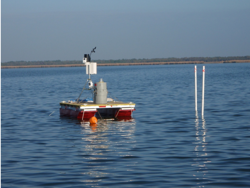
FIGURE 4.3 Photograph of the barge located at LJ28 with deployed ISCO water sampler and Weather Station 1.
