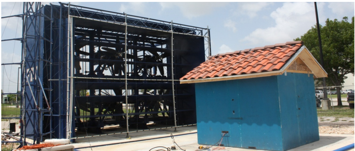
Figure 6.2: Test specimen in front of Wall of Wind at 0° AoA
