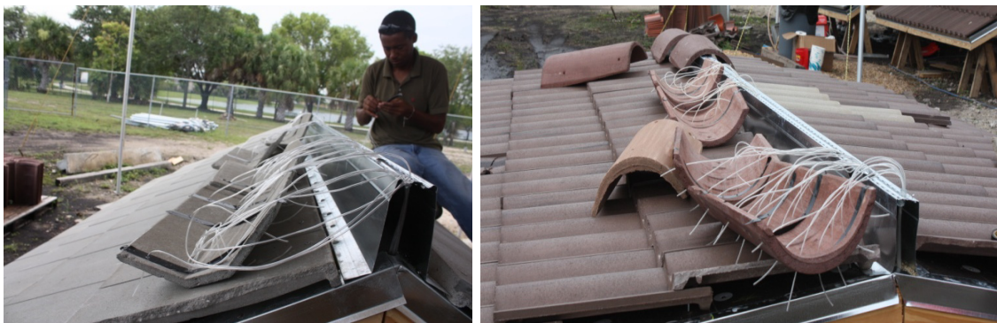
Figure 6.6 Ridge tile Pressure tap distributions: Pressure tap layout along ridge line
