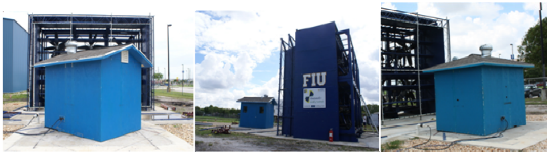
Figure 2.1: Low-rise building with gable and hip roof in front of WoW in a testing position
