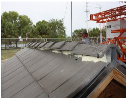
Figure 6.3: Field and ridge tile combinations a) High profile field with barrel ridge tiles; b) Medium profile field with barrel ridge tiles; c) Low profile field with three sided ridge tiles
