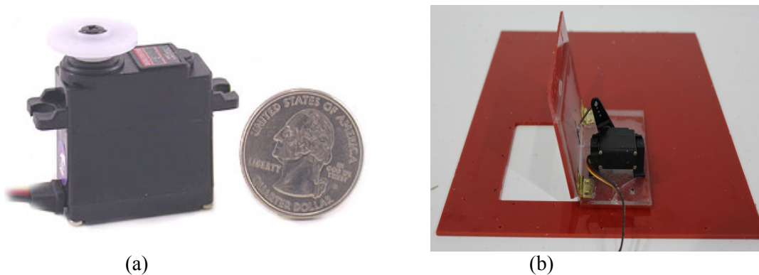
Figure 3.5: Sudden failure simulation technique: a) digital servo motor Hitec HSG-5084MG (Courtesy of ServoCity™), b) window Assembly and Servo in open position.
