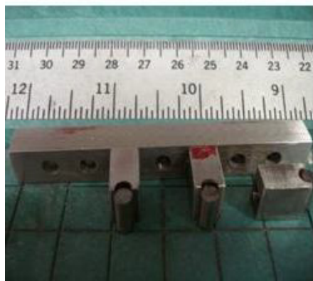
Figure 3.5(e): Loading fixture
