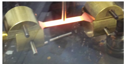
Figure 3.49: Heated electrode showing the central hot zone
