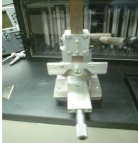
Figure 3.5(a): Fixture used for cutting green laminated tape
