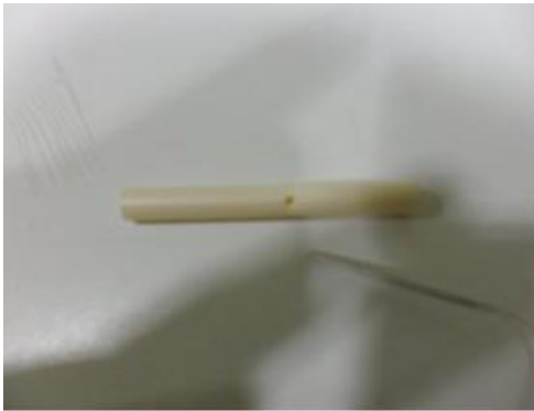
Figure 5.1: Alumina tube with hole drilled to insert thermocouple
