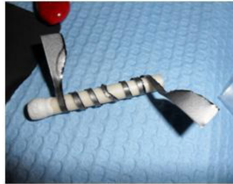
Figure 5.2: Ta sheet wrapped alumina tube
