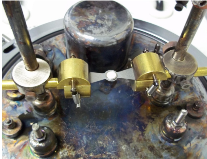
Figure 3.26: JEOL model JEE-4X Thermal evaporator with the Ta electrode and parts to be brazed arranged before brazing
