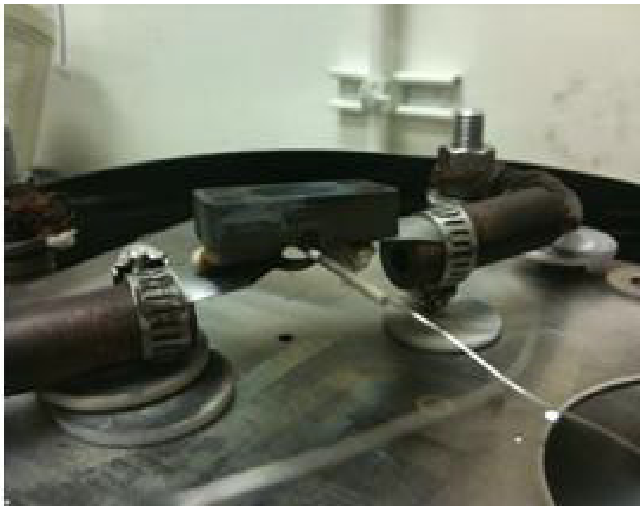
Figure 3.29: Temperature measurement setup of the Ta electrode
