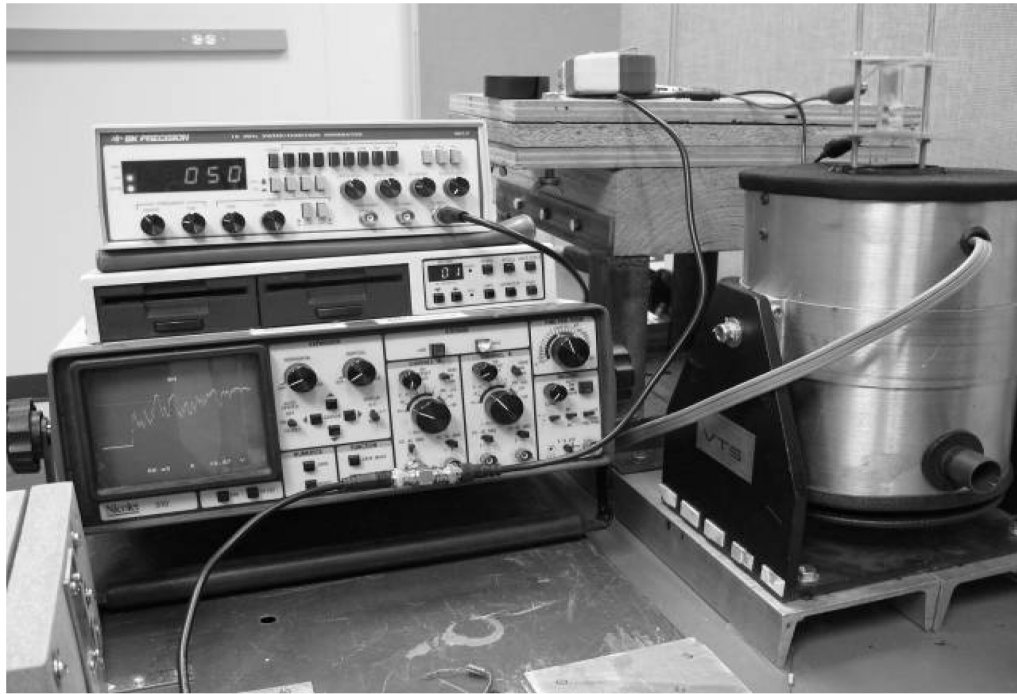
Figure 3.2 Experimental setup used to investigate the electrical response and nonlinear characteristics of piezoelectric actuators
