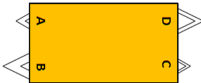
Figure 6: DNPS AFM probe with all four cantilevers.
