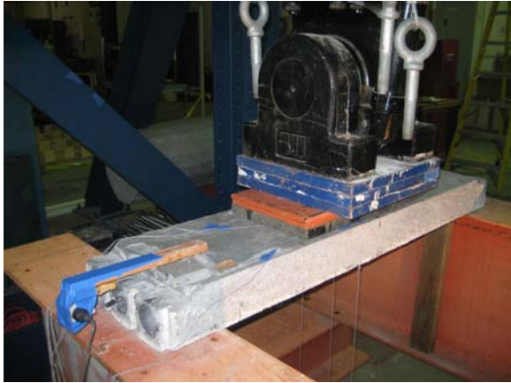
Figure. 6.5 Test Setup for the Uniform Section UHPC-FRP Deck Specimen
