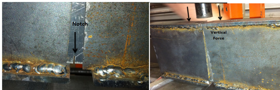
Figure 4.1 Process of crack formation
