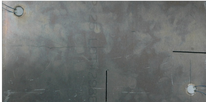
Figure 4.2 Aluminum plate with initial crack.
