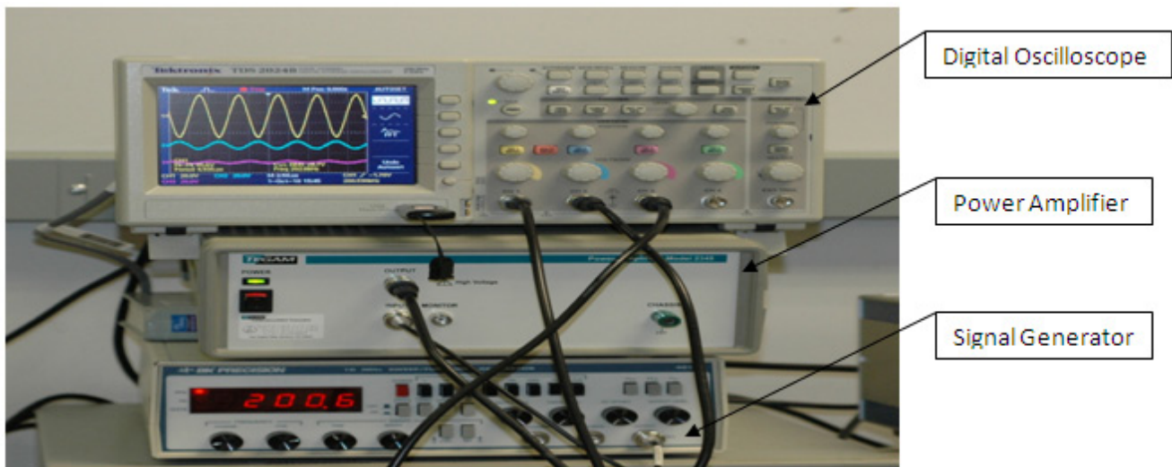
Figure 2.55 – Experimental setup for determining the attenuation of signal over long distance
