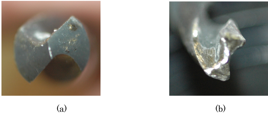
Figure 3.2 – High speed steel drill specimen; (a) new drill and (b) worn out drill
