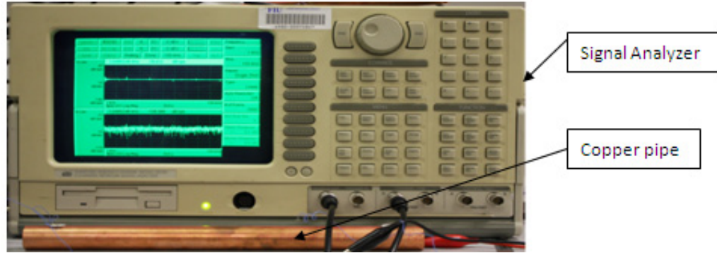
Figure 2.7 – Experimental setup for sweep sine wave method
