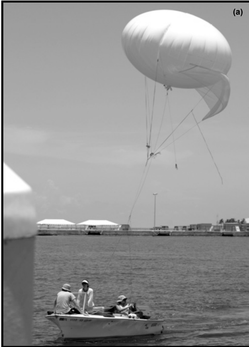
Figure 2. A Floatograph® airship, (a), was used to mount a video camera, (b), for continuous monitoring of dolphin behavior. The airship was tethered to the research vessel and towed during surveys and group sampling.
