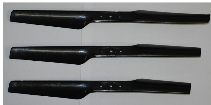
Fig.82 Perfect and Damaged Propellers
