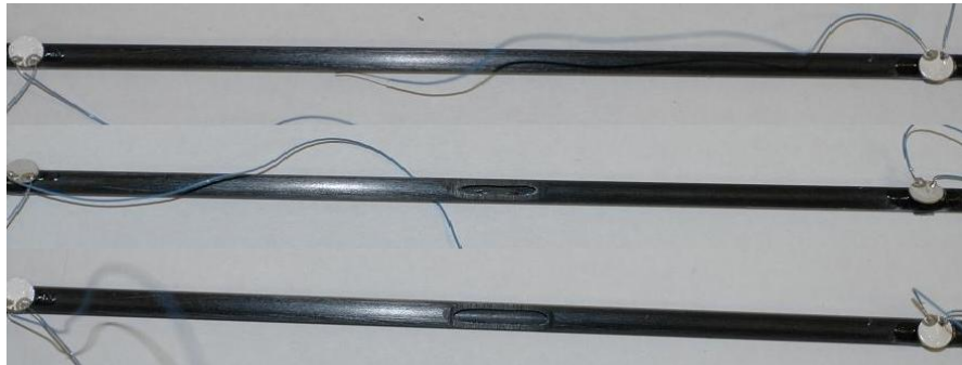
Fig.65 Perfect and Damaged Tubes Bonded with Piezoelectric Actuators and Sensors
