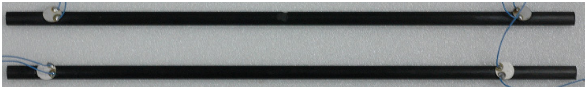
Fig.78 Perfect Tube and Defect Tube with a Notch
