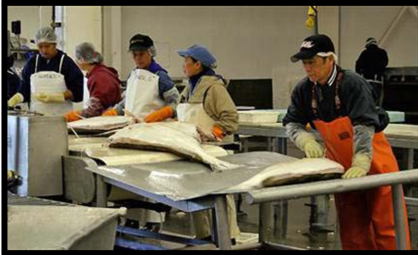
The “slime line”; a term used to describe worker’s gutting the fish in a fish processing plant.
