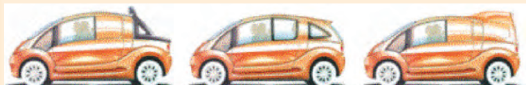
City FlowAIR: Six-seater, family-size compressed air vehicle, not in production yet; planned for US market; estimated 96mph top speed and up to 800 mile range; Compressed Air Engine (CAE) powered and Compressed Air Multiplier (CAM) enabled; three models to choose from.
