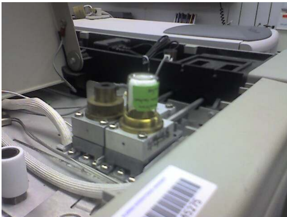
Figure 13: Picture showing collection of human scent compound fractions using a GC/FID
