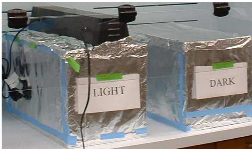
Figure 9: Containers for storage of hand odor samples in the dark and in the presence of UVA/UVB light storage
