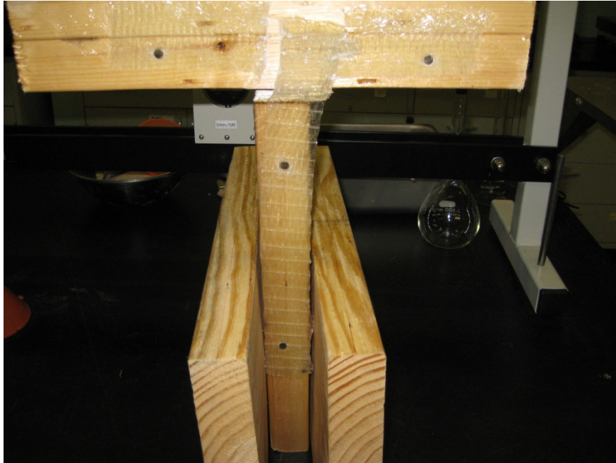
Figure 4-15 Failure mode of configuration-2 (with nails)
