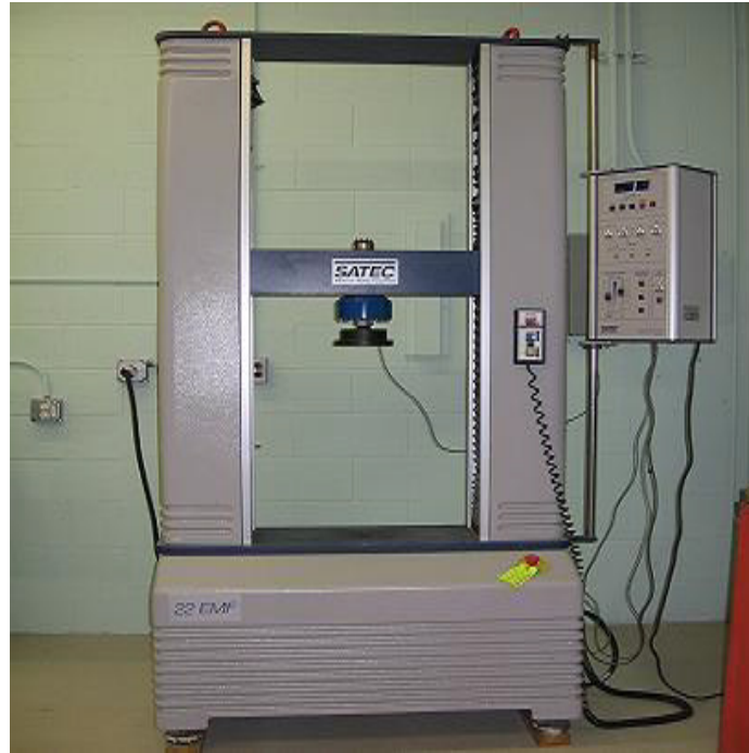
Figure 3-3 Universal Testing Machine with 22 kip capacity (Model Mark III, 22 EMF)
