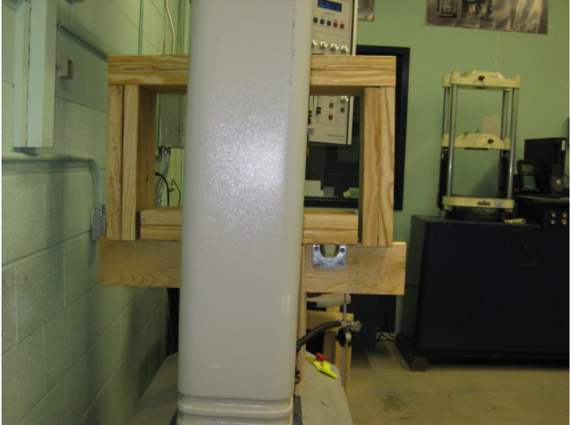
Figure 4-10 Test setup for gable end connection
