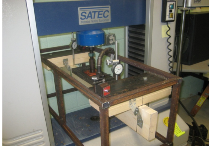
Figure 3-4 Experimental setup for testing clips using SPF and SYP wood types
