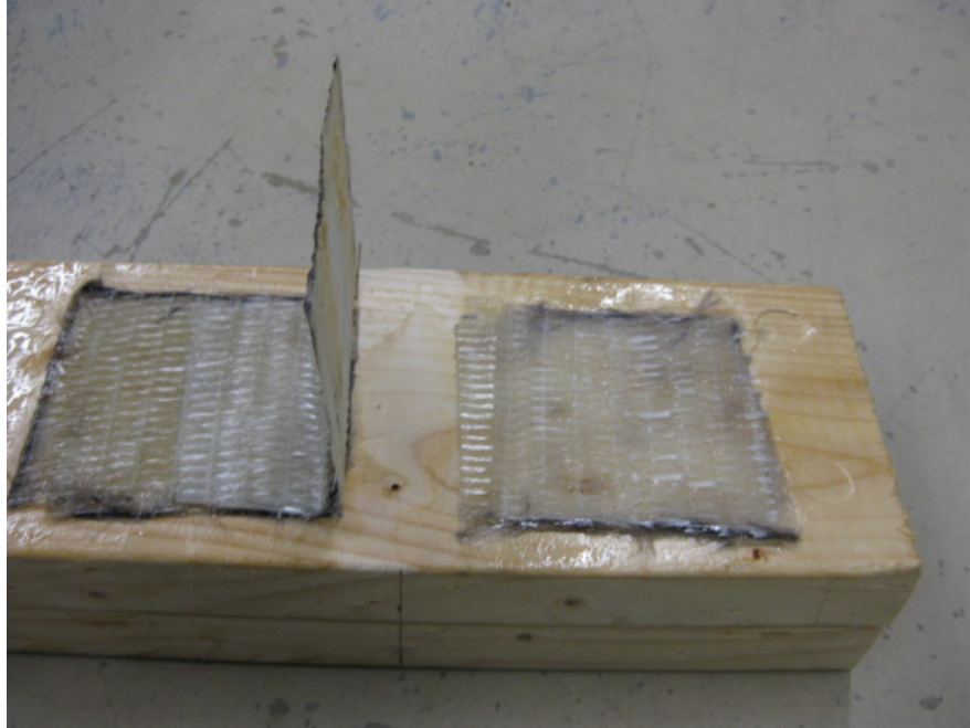
Figure 4-13 Failure mode of configuration-4
