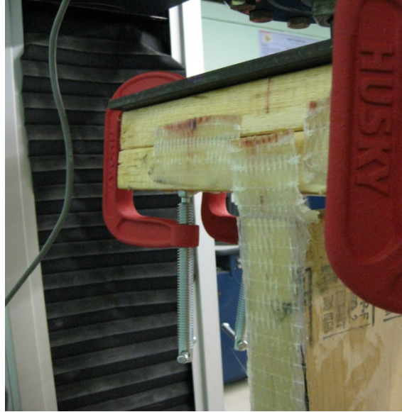
Figure 4-12 Failure mode of configuration-2
