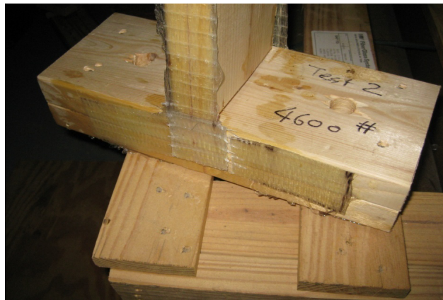
Figure 5-2 Mode of failure for stud to top plate connection
