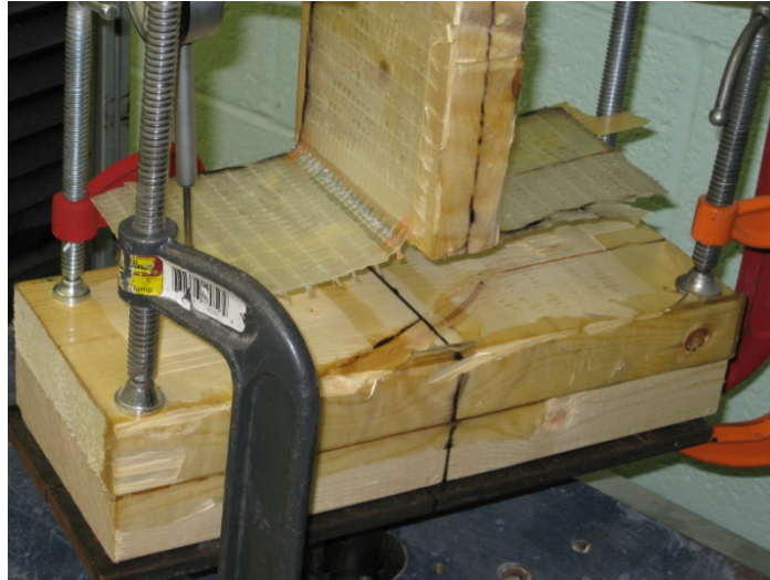
Figure 4-11 Failure mode of Configuration-1
