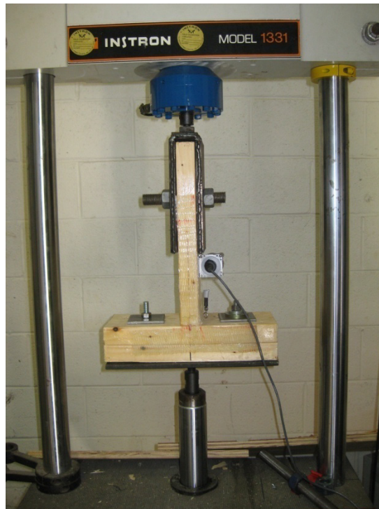
Figure 4-7 Test setup for stud to top plate connection
