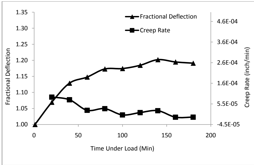
Figure 5-16 Fractional deflection and Creep rate graph for 75% stress ratio (Test-1) for Gable end connection
