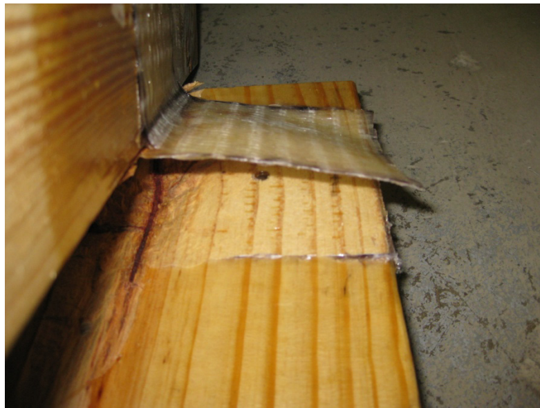
Figure 4-16 Failure mode of configuration-1
