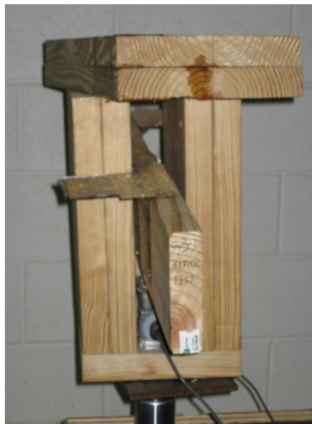
Figure 5-3 Failure mode of Gable end connection
