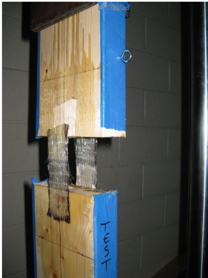
Figure 5-1 Failure mode of shear connection test.
