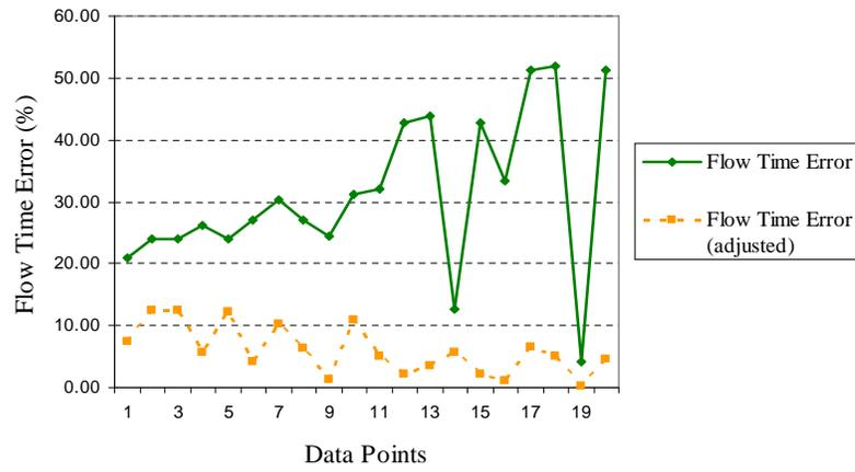
Figure 4.37: Flow time error for five product instances using correction factors in the  $E_2 - E_2$  case.
