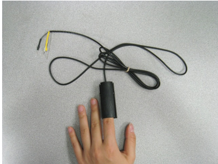
Figure 4-15: BVP sensor -PPG (UFI Model 1020)
