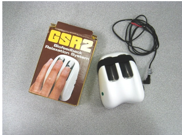
Figure 4-13: GSR2 module for GSR measurement system
