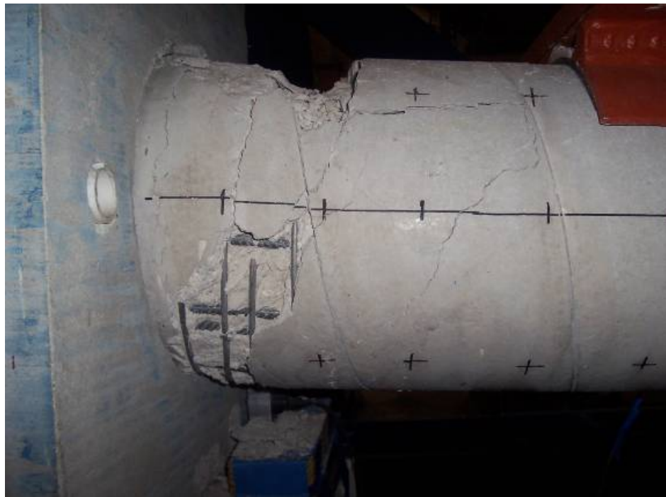
Figure 4.12 East View of Final Cracking Pattern Close to Footing in Specimen RC
