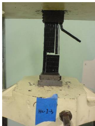
Figure 5.49 Failure Mode of HC-I-3: SGM
