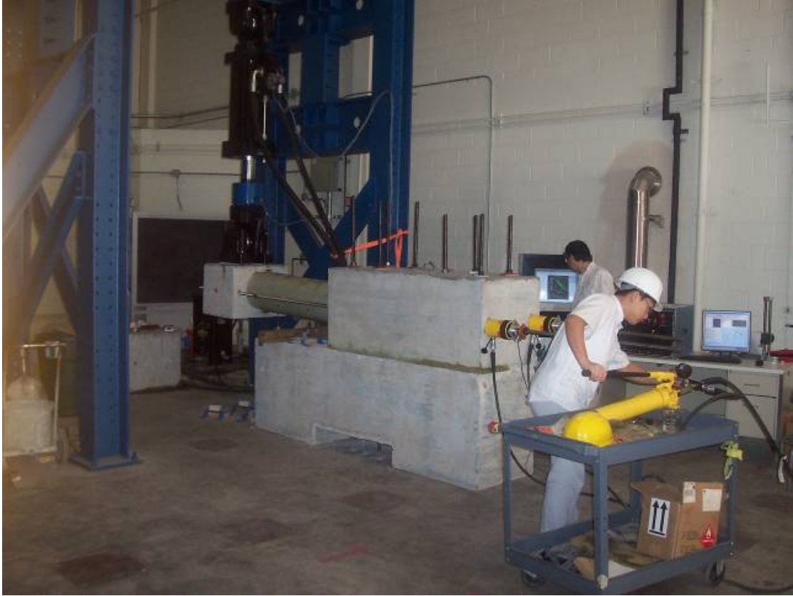
Figure 3.26 Post-Tensioning of Specimen G to Simulate Axial Force
