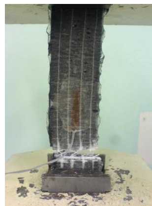
Figure 5.62 Failure Mode of HL-V-2: LWB
