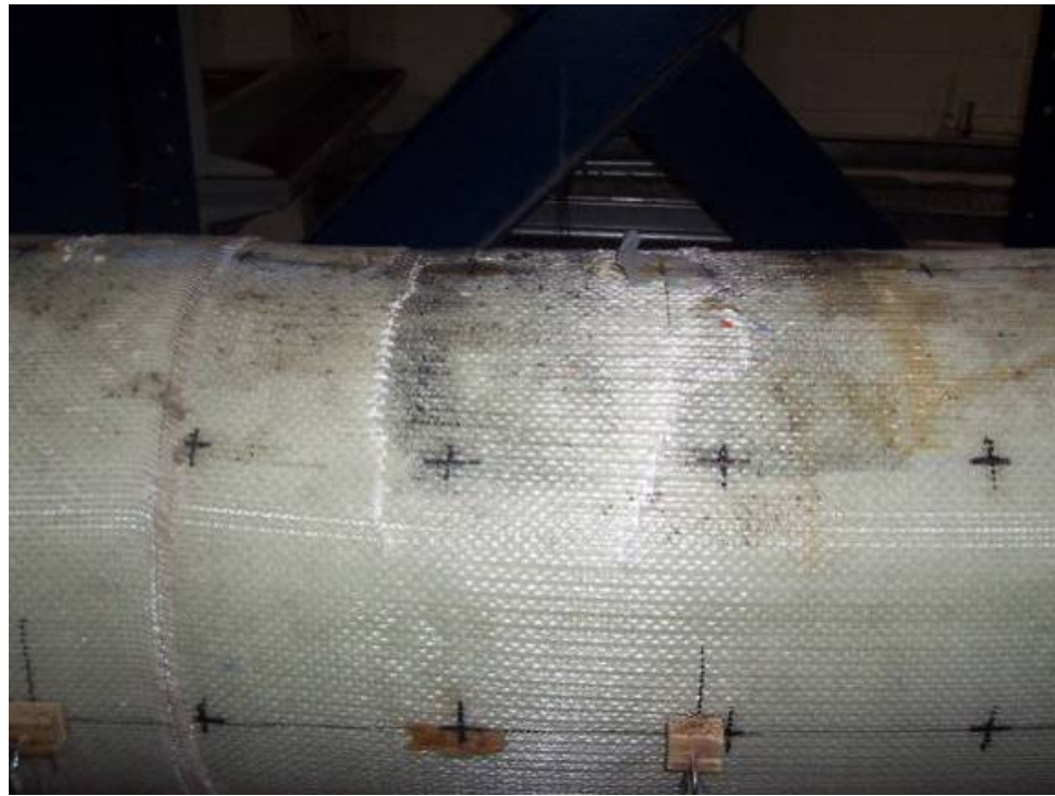
Figure 4.16 Cracking Pattern of Specimen G (East View)
