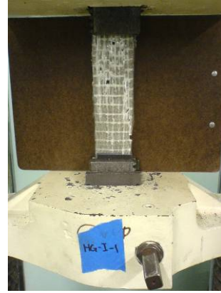
Figure 5.52 Failure Mode of HG-I-1: SGM
