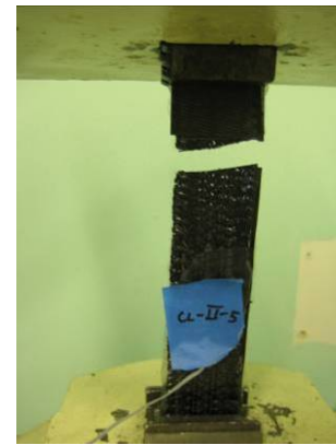
Figure 5.24 Failure Mode of CL-II-5: LAT
