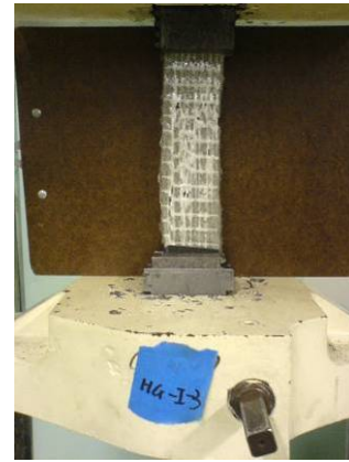
Figure 5.54 Failure Mode of HG-I-3: SGM
