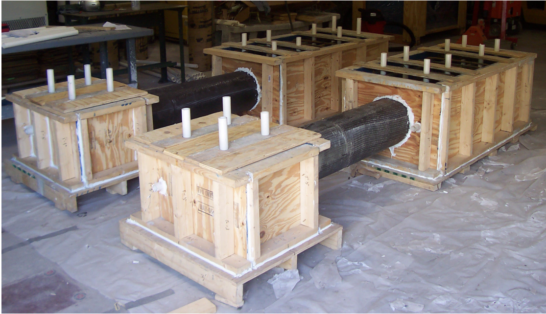
Figure 3.9 Formworks of Specimens H and SC
