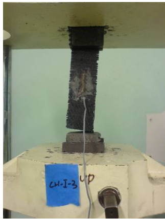
Figure 5.5 Failure Mode of CH-I-3: LWV
