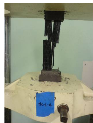
Figure 5.50 Failure Mode of HC-I-4: SGM
