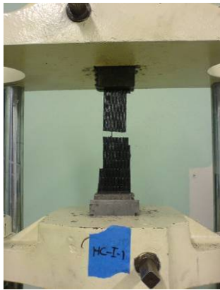
Figure 5.47 Failure Mode of HC-I-1: LGM
