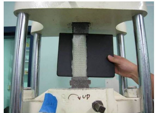
Figure 5.32 Failure Mode of GH-III-5: OAT
