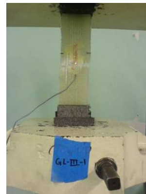
Figure 5.44 Failure Mode of GL-III-1': LGM
