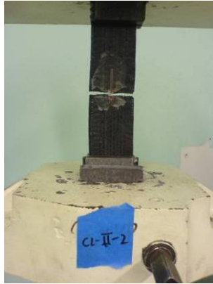
Figure 5.21 Failure Mode of CL-II-2: LGM
