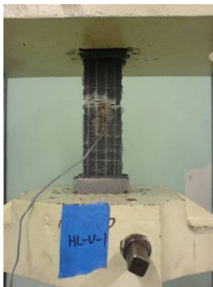
Figure 5.61 Failure Mode of HL-V-1: LGM
