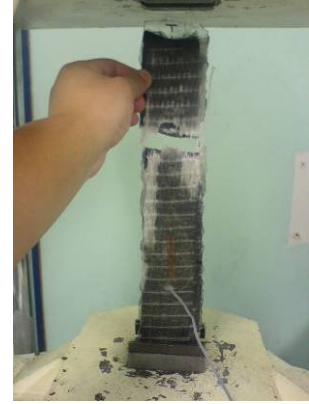
Figure 5.58 Failure Mode of HH-V-2: LAT
