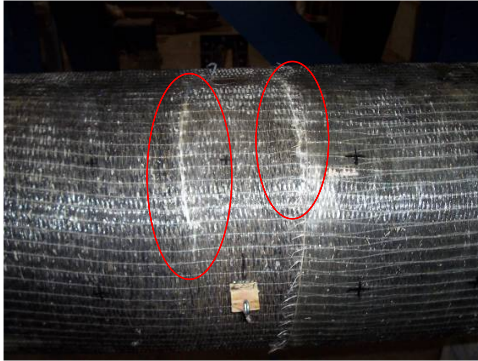
Figure 4.21 Crumpling Crack in Specimen H at the Top (East View)
