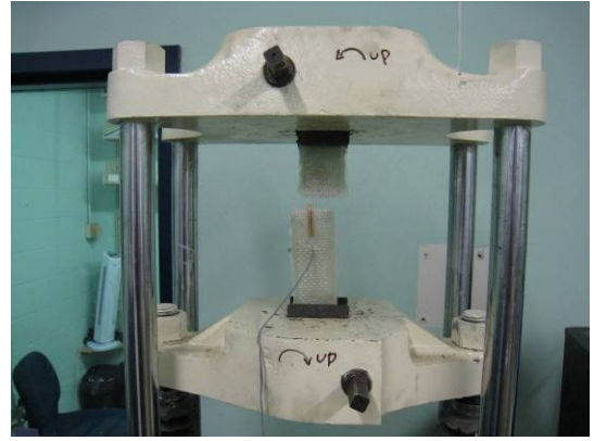
Figure 5.28 Failure Mode of GH-III-1: LGM
