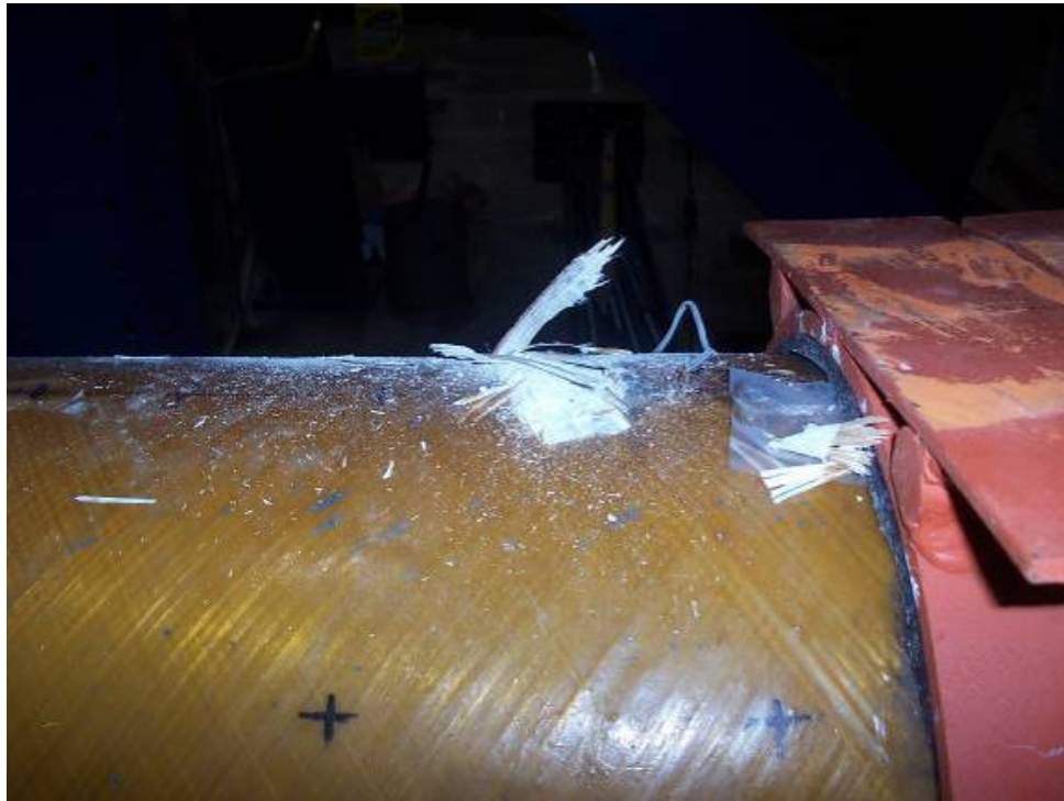
Figure 4.14 Crushing of Specimen Y at the Top (East View)
