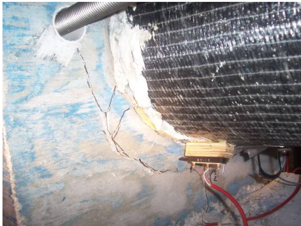
Figure 3.39 Splitting of Concrete Footing in Specimen H
