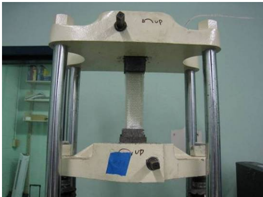
Figure 5.31 Failure Mode of GH-III-4: LAB
