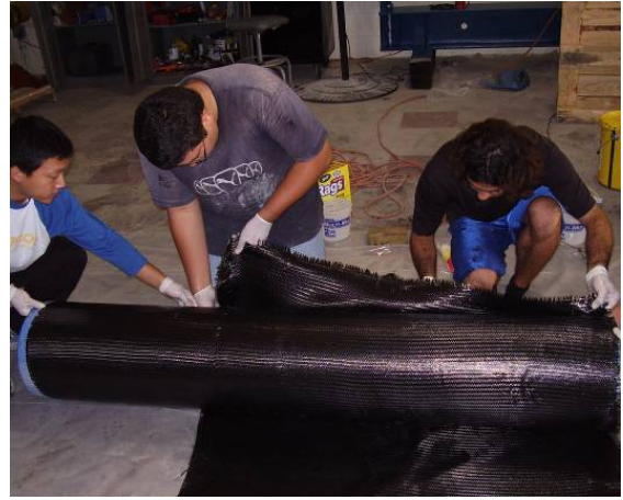
Figure 3.2 Preparation of Carbon FRP Tube in the Laboratory
