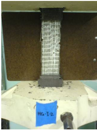
Figure 5.53 Failure Mode of HG-I-2: SGM
