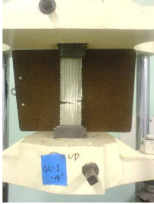
Figure 5.39 Failure Mode of GL-I-4': LGM
