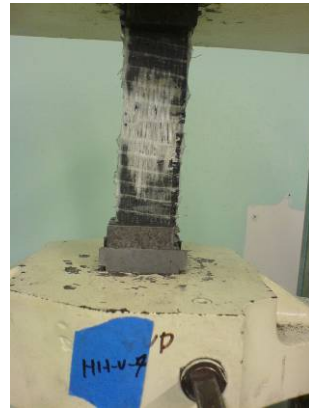
Figure 5.60 Failure Mode of HH-V-4: LGM
