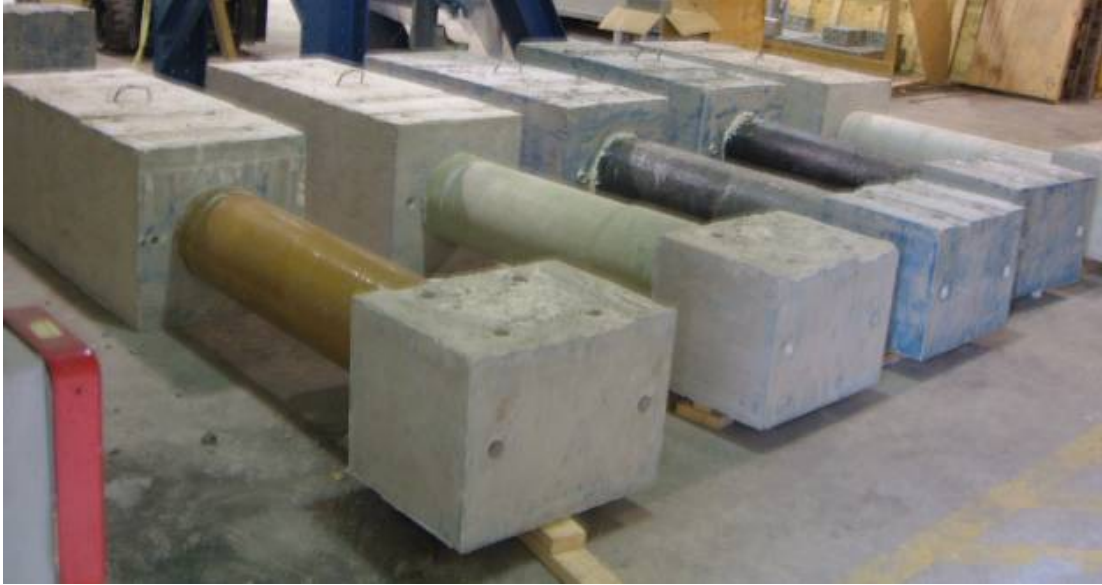
Figure 3.13 Five Short Column Specimens after De-Molding
