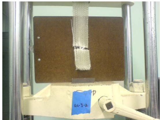
Figure 5.37 Failure Mode of GL-I-2': LAB
