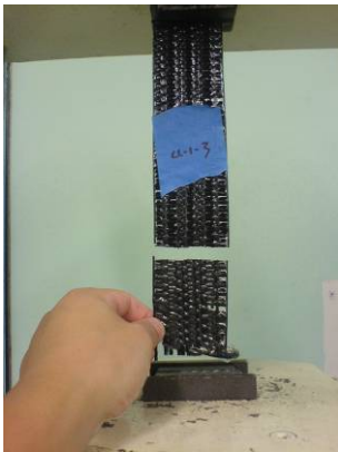
Figure 5.17 Failure Mode of CL-I-3: LIB
