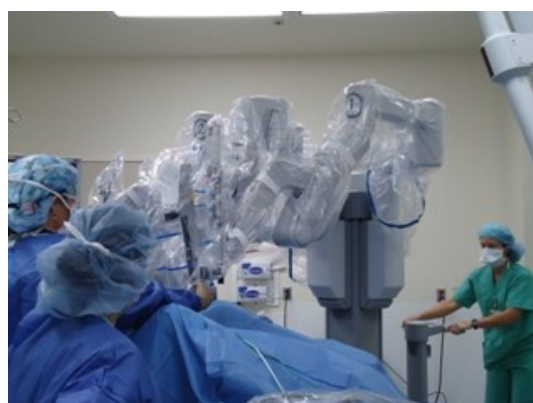
Figure 3: Lateral docking of the draped Robot.
