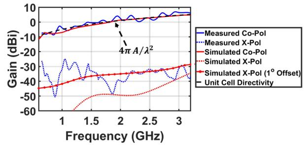
**FIGURE 8.** Measured vs simulated broadside co-polarized and cross-polarized gain of the center element as a function of frequency. For comparison with measurements, the simulated case of  $1^\circ$  misalignment in  $\phi$  is also given, along with maximum achievable gain.
