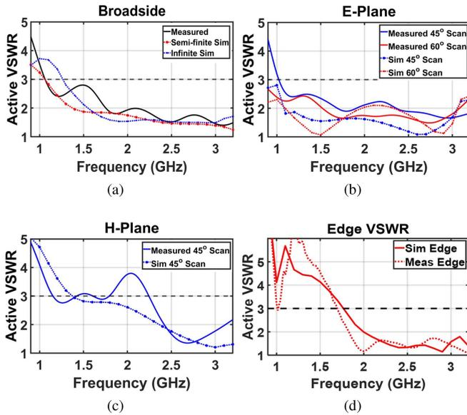
**FIGURE 7.** Measured active VSWR of an embedded center array element for (a) broadside, (b) E-Plane, (c) H-Plane scanning cases with comparisons to simulation, and (d) edge elements measured active VSWR at broadside.
