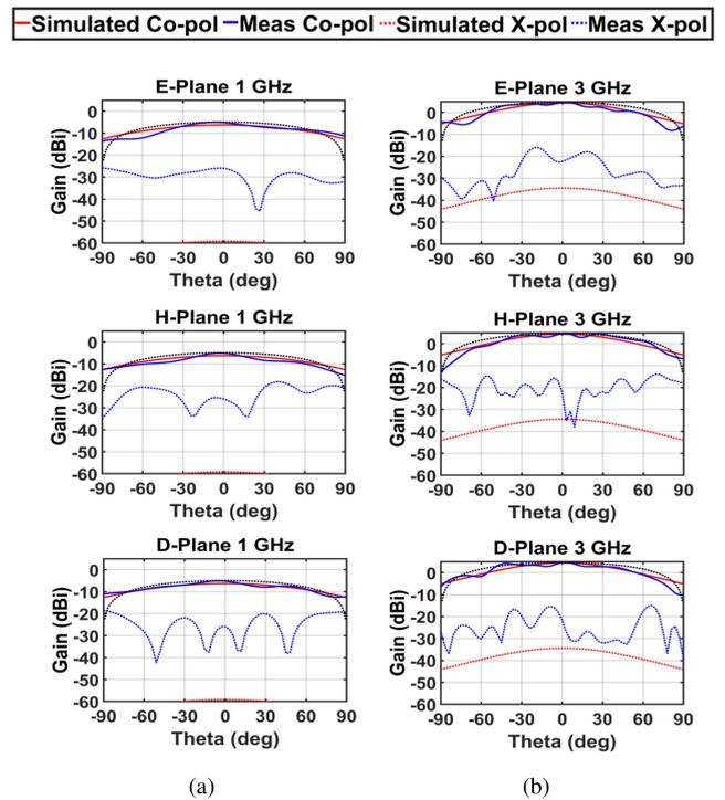
**FIGURE 9.** Measured embedded patterns of the center element in the E, H and D-planes for (a) 1 GHz, and (b) 3 GHz. Comparisons to simulation are also given. More than 20 dB polarization purity is achieved out to  $\theta = \pm 60^\circ$ .
