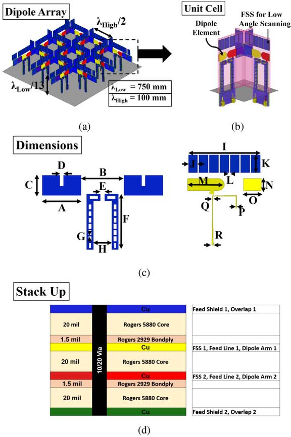
**FIGURE 1.** Pictorial representation of (a) the dual-polarized dipole array and (b) its infinite array unit cell. The (c) dimensions of the design and (d) a printed circuit board stack-up (color coded) are also given to show the layer details.
