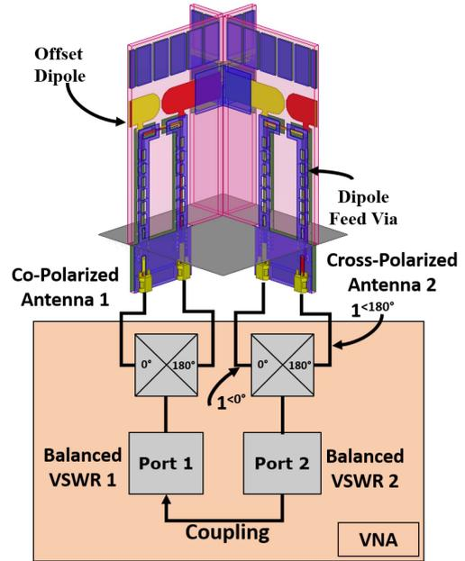
**FIGURE 6.** Measurement setup employed to characterise balanced S-parameters using the 4-port VNA. Note: For gain measurements, an external Marki Bal-0003 balun was used to translate the differential antenna port to the single-ended measurement port.
