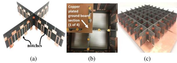
**FIGURE 5.** (a) Fabricated  $8 \times 1$  antenna strip being assembled as an egg-crate, (b) Feed ports for four antenna elements on the bottom side on the fabricated array, and (c) Fully assembled  $8 \times 8$  dipole array on  $384\text{mm} \times 384\text{mm}$  ground plan.
