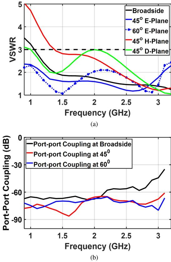
**FIGURE 4.** (a) Simulated infinite array active VSWR in the E, H, and D-planes of the dipole array at various scan angles, (b) Simulated unit cell H-pol to V-pol (port-to-port) coupling for different scan cases.
