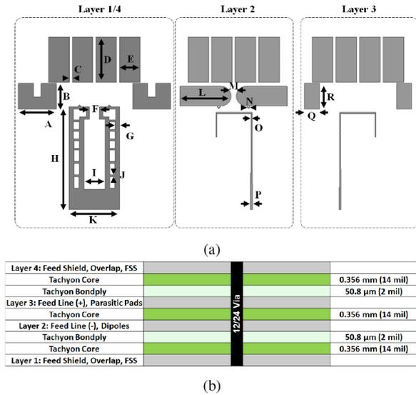
**FIGURE 7.** (a) Unit cell details of the designed dual-polarized D-TCDA. The (b) antenna stack-up shows the mirrored metal layers are printed on 0.36mm (14 mil) substrate layers with relative dielectric constant of  $\epsilon_r = 3.0$ .
