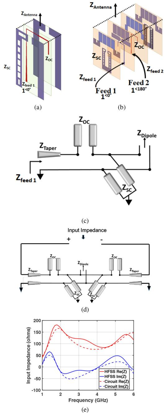
**FIGURE 4.** Marchand baluns for TCDA: (a) Marchand balun sketch, (b) BWIT sketch, (c) behavioral circuit model, (d) BWIT behavioral circuit model, (e) BWIT impedance profile. The behavioral model is verified by its close relation to the full-wave impedance profile.
