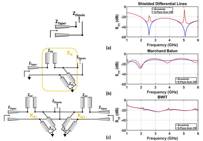
**FIGURE 6.** Transmission line equivalent circuits and  $S_{11}$  performance for three different feeds: (a) Basic differential lines, (b) Marchand Balun and (c) BWIT at broadside (red) and with a common mode excitation (blue).
