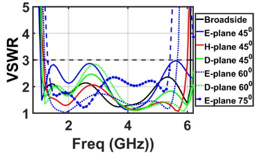
**FIGURE 9.** Simulated infinite array VSWR in the E, H, and D-planes of the single-polarized array. Broadside and scanning VSWR at 45° and 60° are shown.
