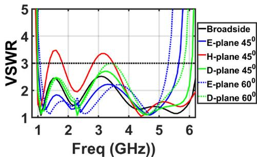
**FIGURE 8.** Simulated infinite array VSWR in the E, H, and D-planes of the dual-polarized array at broadside and scanning to 60° in the E/D-planes and 45° in the H-plane.
