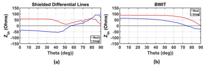
**FIGURE 3.** Infinite array simulations at the common mode resonant frequencies in Fig. 2 showing input impedance versus scan angle. Specifically (a) shielded twin lines at 3.6 GHz, and (b) BWIT feed at 2.2 GHz. The impedance values imply that the discontinuity in the shielded twin lines are a near-short at resonance and the BWIT is unaffected.
