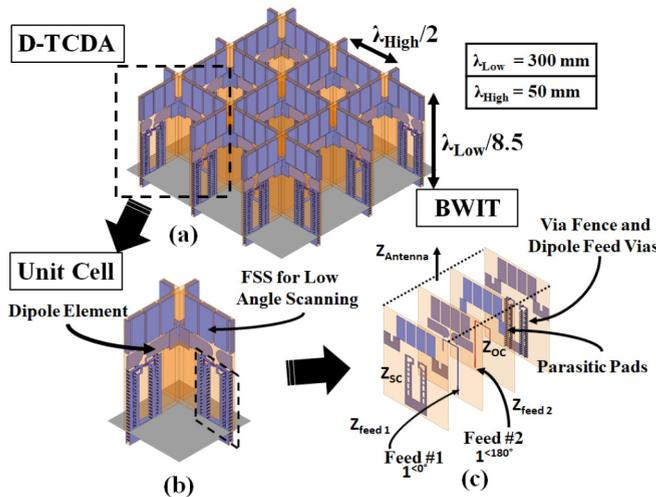
**FIGURE 1.** Pictorial representation of a (a) dual polarized differential TCDA (D-TCDA) array with (b) unit cell of dual offset D-TCDA design, along with the (c) improved BWIT differential matching network.
