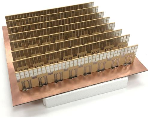
FIGURE 10. Fabricated 8x8 single-polarized D-TCDA placed on a 22.86cmx22.86cm ground plane.
