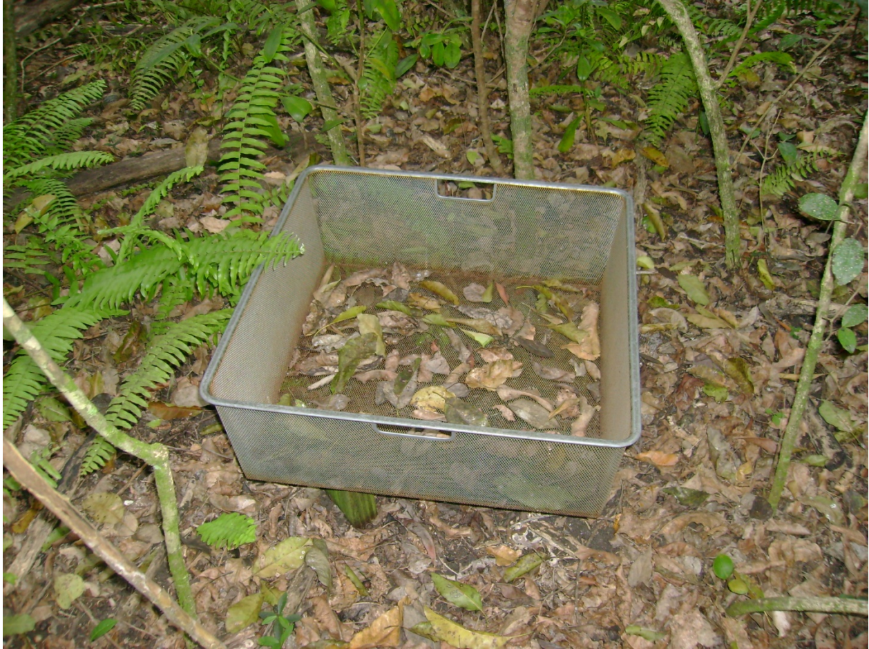
Plate 1: Epoxy-coated steel wire fine-mesh (52.70 x 52.70 x 18.42 cm) litter traps used in the three high frequency sampling tree islands.
