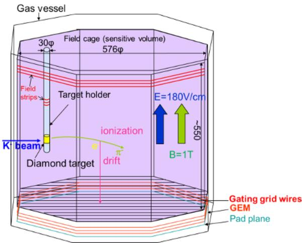
Figure 2. Schematic view of HypTPC.
