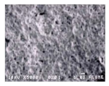
Figure A-2. Micrograph of silver metallo-organic surface coating on DuPont 951AT (LTCC).
