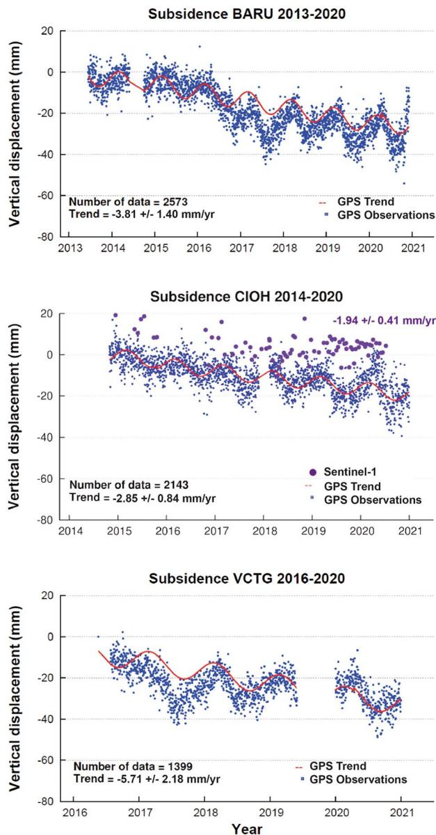
**Figure 3.** Time series (2013–2020) of subsidence (mm) at three GPS geodetic stations (Fig. 1c) in Cartagena (Data from the GeoRED Project, Space Geodesy Research Group of the Colombian Geological Survey-CGS, Servicio Geológico Colombiano). Sentinel-1 vertical displacement observations (mm) during the 2014–2020 period are plotted (purple) at the GPS-tide gauge station (CIOH) (center). GPS time series generated by GNUPLOT v 4.2 (<http://www.gnuplot.info/>).
