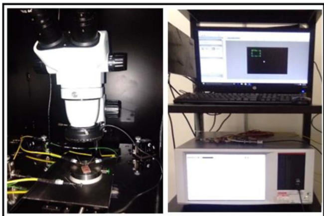
Figure 8. The pH sensor characteristics measurement setup using Keithley 4200 semiconductor characterization system.
